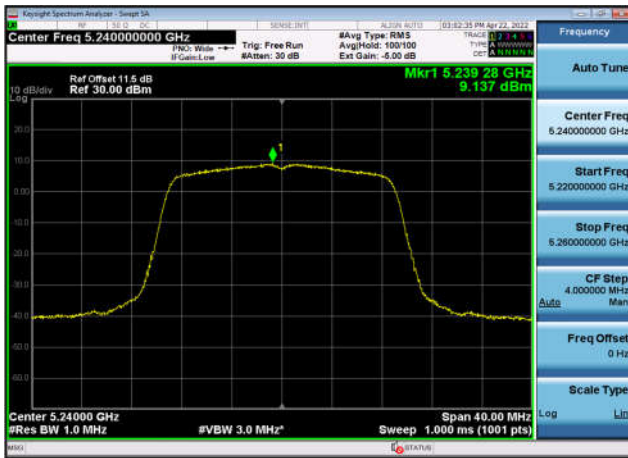
U-NII-1 Power spectral density-802.11 ac(40MHz),5230MHz,Ant1
