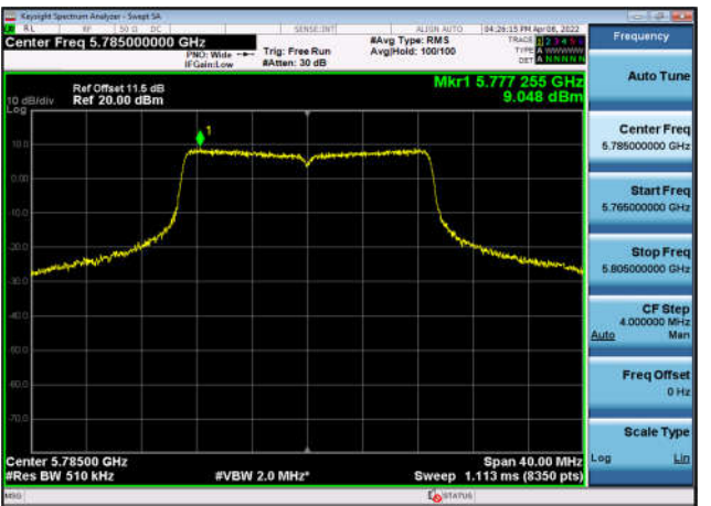
U-NII-3 Power spectral density-802.11 n(40MHz),5755MHz,Ant1
