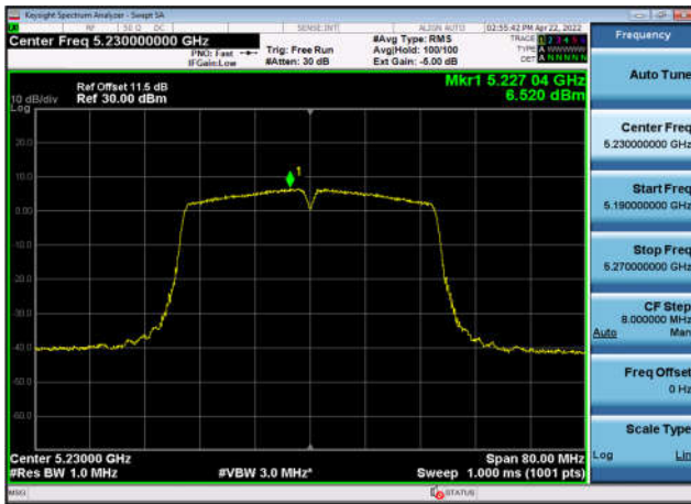
U-NII-1 Power spectral density-802.11 a(20MHz),5220MHz,Ant1
