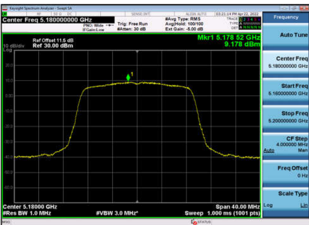
U-NII-1 Power spectral density-802.11 n(20MHz),5180MHz,Ant1
