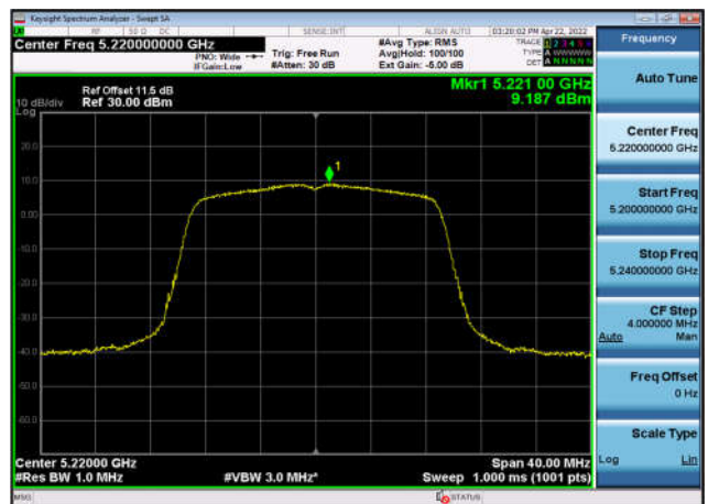
U-NII-1 Power spectral density-802.11 n(20MHz),5220MHz,Ant1
