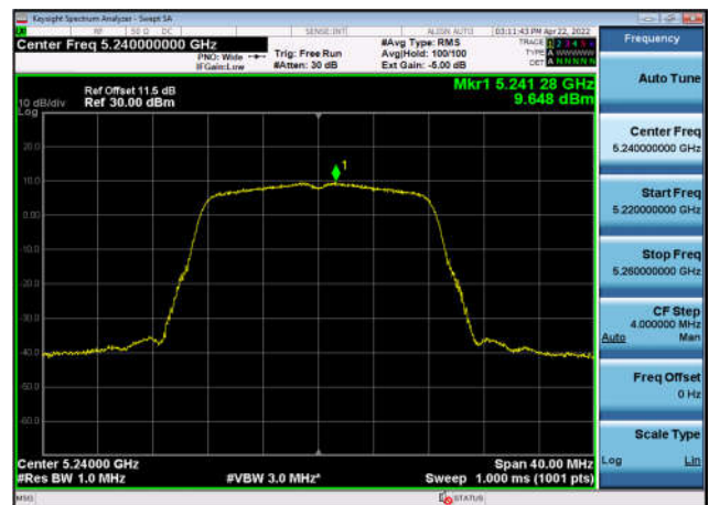
U-NII-1 Power spectral density-802.11 a(20MHz),5240MHz,Ant1
