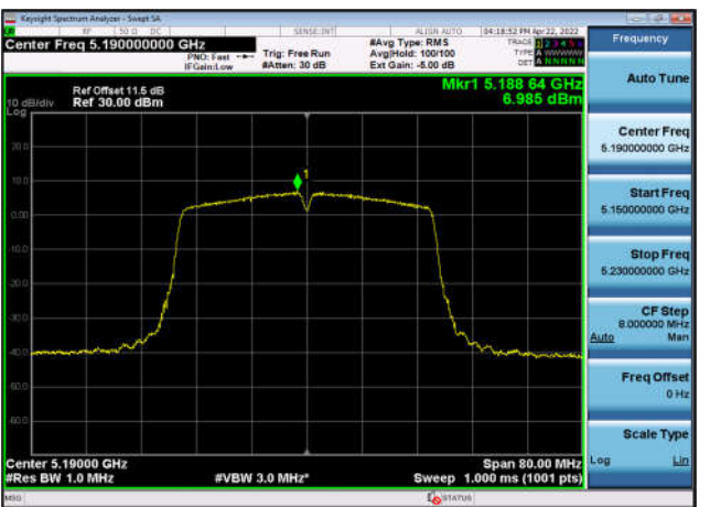
U-NII-1 Power spectral density-802.11 n(40MHz),5190MHz,Ant1
