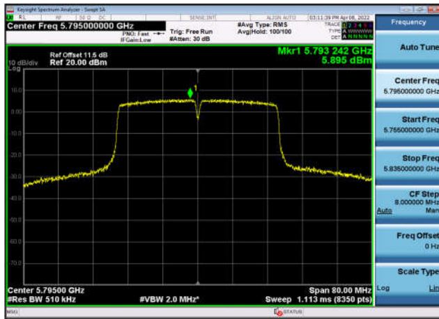
U-NII-3 Power spectral density-802.11 ax(20MHz),5745MHz,Ant0
