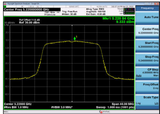
U-NII-1 Power spectral density-802.11 ac(40MHz),5190MHz,Ant1
