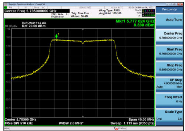
U-NII-3 Power spectral density-802.11 ax(40MHz),5755MHz,Ant0
