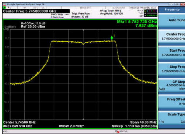
U-NII-3 Power spectral density-802.11 ax(20MHz),5825MHz,Ant0
