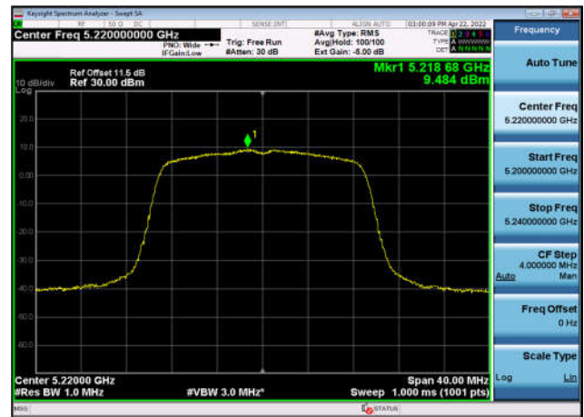
U-NII-1 Power spectral density-802.11 n(40MHz),5190MHz,Ant1
