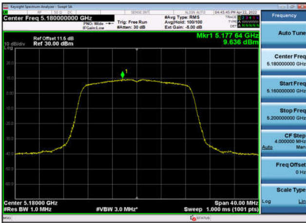
U-NII-1 Power spectral density-802.11 ac(20MHz),5240MHz,Ant1
