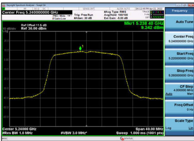
U-NII-1 Power spectral density-802.11 n(20MHz),5240MHz,Ant1
