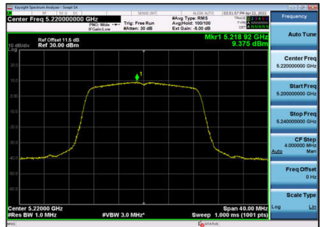
U-NII-1 Power spectral density-802.11 ac(20MHz),5220MHz,Ant1
