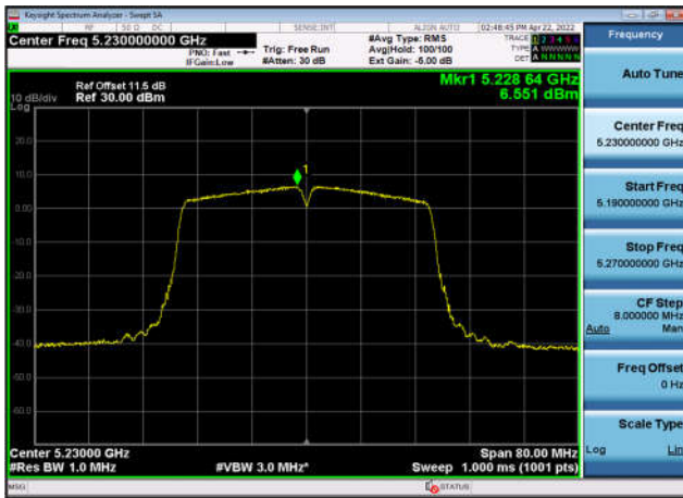
U-NII-1 Power spectral density-802.11 ax(20MHz),5180MHz,Ant1
