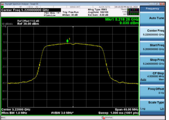
U-NII-1 Power spectral density-802.11 n(40MHz),5190MHz,Ant1
