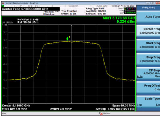
U-NII-1 Power spectral density-802.11 ac(20MHz),5240MHz,Ant1
