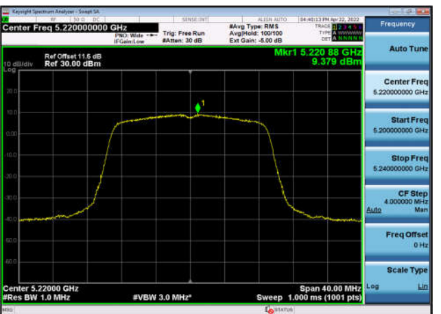
U-NII-1 Power spectral density-802.11 n(20MHz),5220MHz,Ant1
