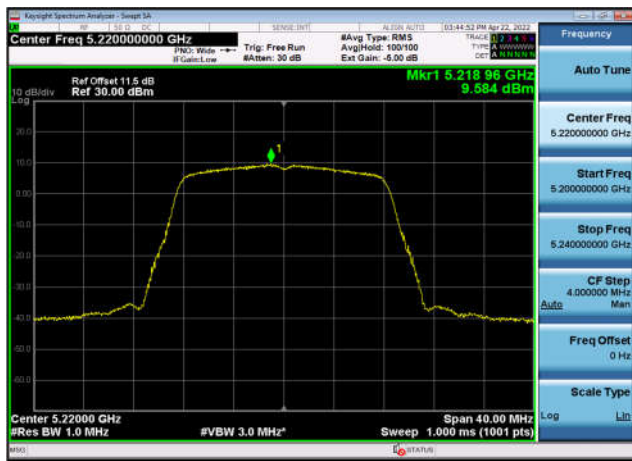
U-NII-1 Power spectral density-802.11 ac(20MHz),5180MHz,Ant1
