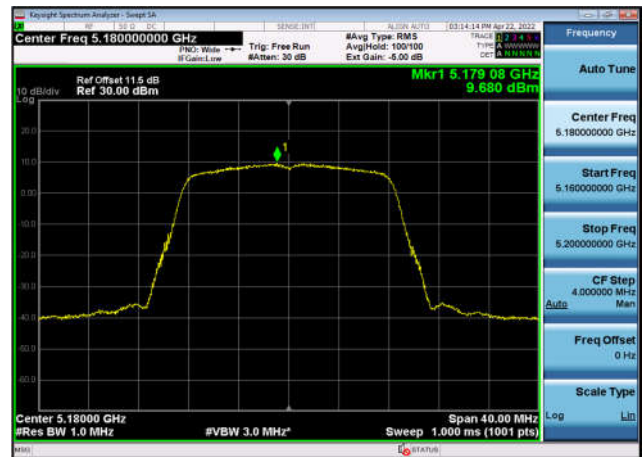
U-NII-1 Power spectral density-802.11 a(20MHz),5240MHz,Ant1
