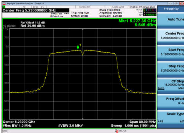
U-NII-1 Power spectral density-802.11 a(20MHz),5220MHz,Ant1
