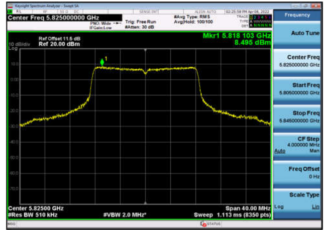
U-NII-3 Power spectral density-802.11 ac(20MHz),5785MHz,Ant0
