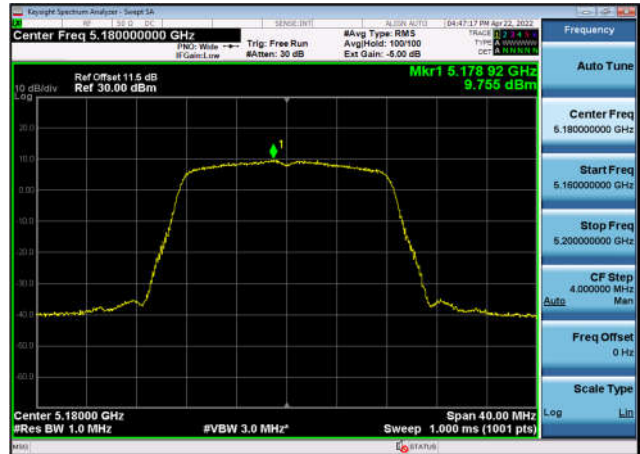
U-NII-1 Power spectral density-802.11 a(20MHz),5240MHz,Ant1
