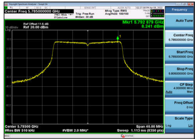
U-NII-3 Power spectral density-802.11 n(40MHz),5755MHz,Ant0
