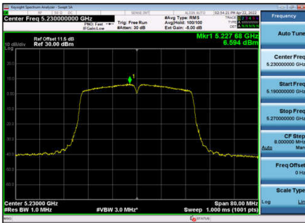
U-NII-1 Power spectral density-802.11 ax(20MHz),5180MHz,Ant1
