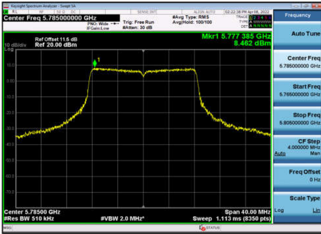
U-NII-3 Power spectral density-802.11 ac(20MHz),5745MHz,Ant0
