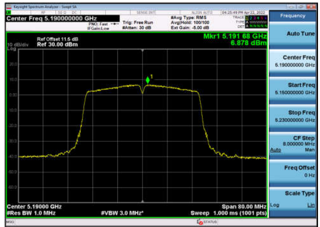
U-NII-1 Power spectral density-802.11 ac(80MHz),5210MHz,Ant1
