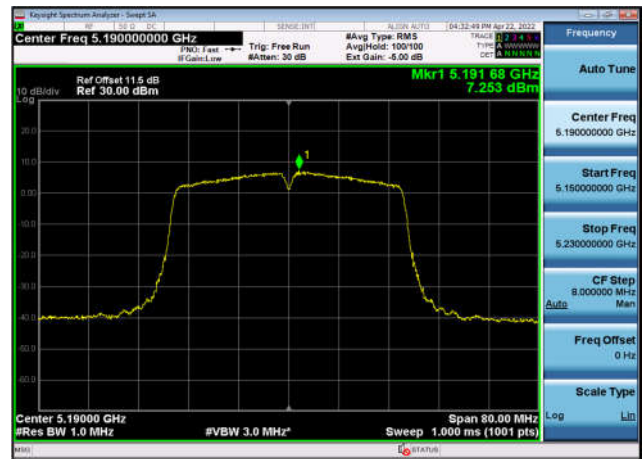
U-NII-1 Power spectral density-802.11 ac(80MHz),5210MHz,Ant1
