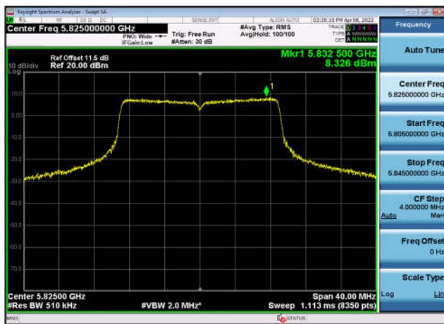
U-NII-3 Power spectral density-802.11 ax(20MHz),5825MHz,Ant0
