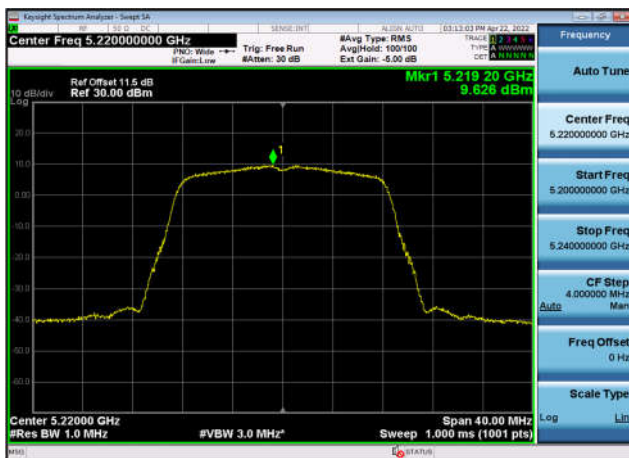
U-NII-1 Power spectral density-802.11 a(20MHz),5220MHz,Ant1
