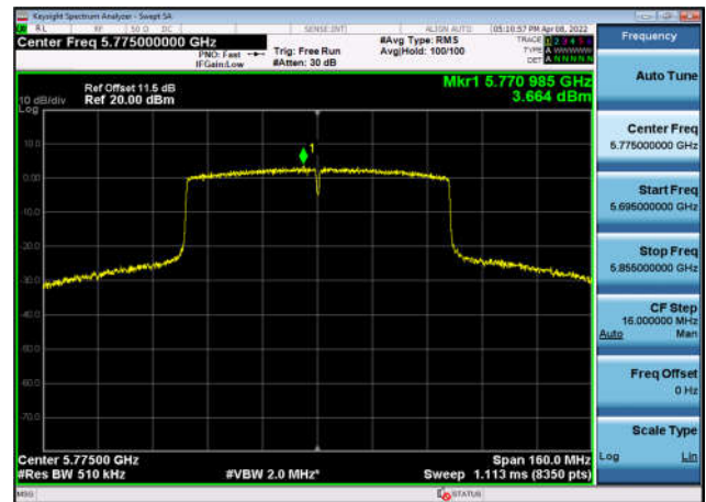
U-NII-3 Power spectral density-802.11 ax(20MHz),5785MHz,Ant1
