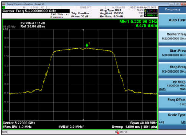
U-NII-1 Power spectral density-802.11 ac(20MHz),5180MHz,Ant1
