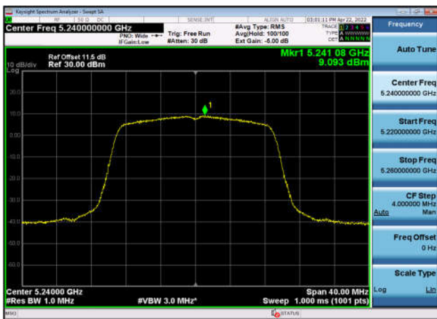
U-NII-1 Power spectral density-802.11 n(20MHz),5240MHz,Ant1
