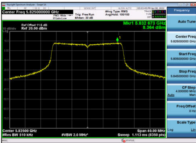
U-NII-3 Power spectral density-802.11 ac(20MHz),5825MHz,Ant0
