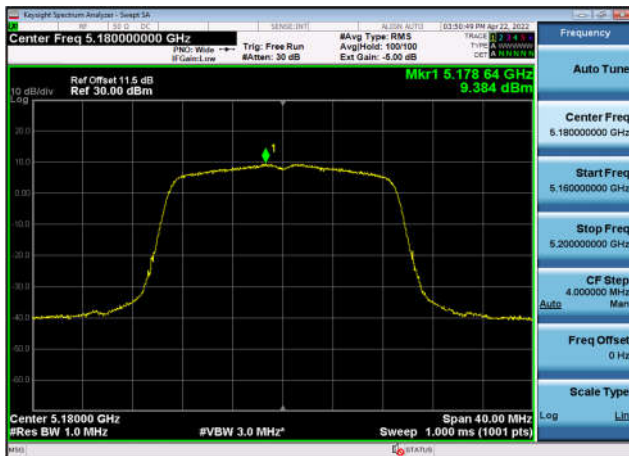
U-NII-1 Power spectral density-802.11 ac(20MHz),5180MHz,Ant1
