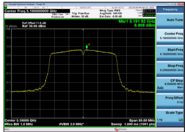
U-NII-1 Power spectral density-802.11 a(20MHz),5180MHz,Ant1
