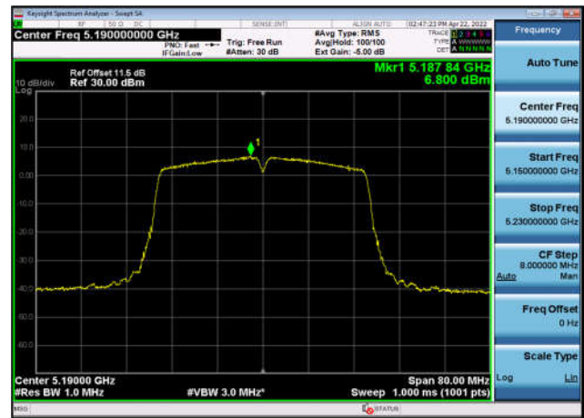
U-NII-1 Power spectral density-802.11 ac(40MHz),5190MHz,Ant1
