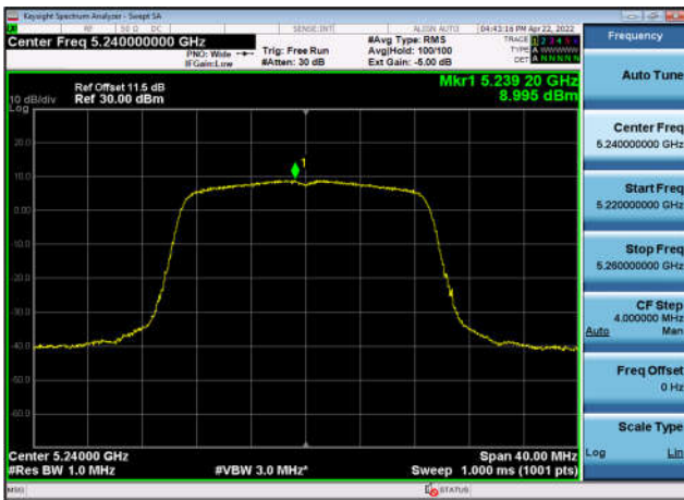
U-NII-1 Power spectral density-802.11 ac(40MHz),5230MHz,Ant1
