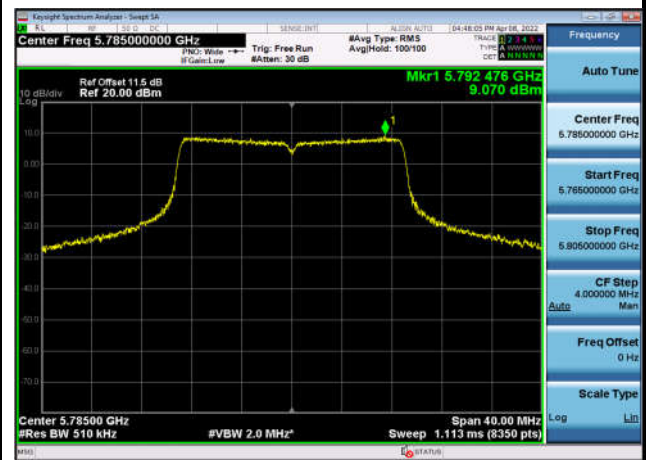
U-NII-3 Power spectral density-802.11 ac(20MHz),5785MHz,Ant1
