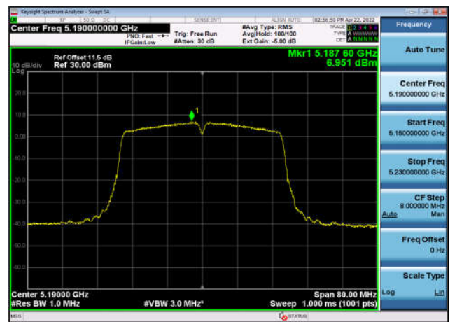
U-NII-1 Power spectral density-802.11 n(40MHz),5190MHz,Ant1
