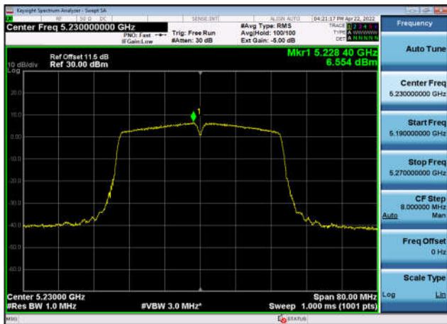
U-NII-1 Power spectral density-802.11 ax(20MHz),5180MHz,Ant1
