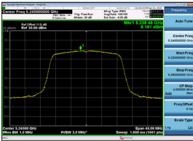
U-NII-1 Power spectral density-802.11 ac(20MHz),5240MHz,Ant1
