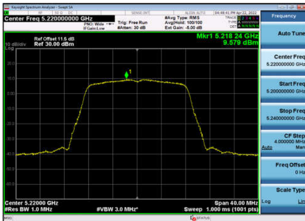
U-NII-1 Power spectral density-802.11 a(20MHz),5220MHz,Ant1
