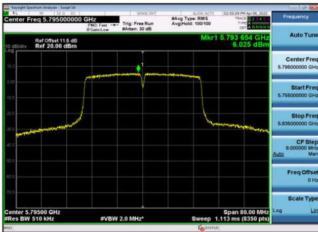
U-NII-3 Power spectral density-802.11 n(40MHz),5795MHz,Ant0
