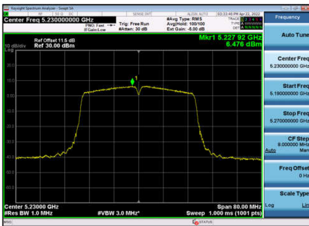
U-NII-1 Power spectral density-802.11 a(20MHz),5220MHz,Ant1
