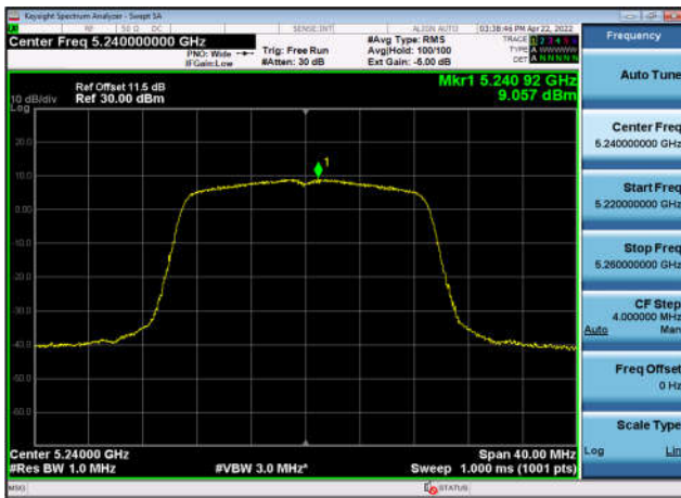
U-NII-1 Power spectral density-802.11 n(40MHz),5230MHz,Ant1
