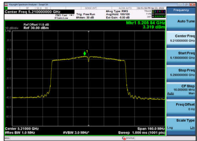
U-NII-1 Power spectral density-802.11 ax(20MHz),5220MHz,Ant1
