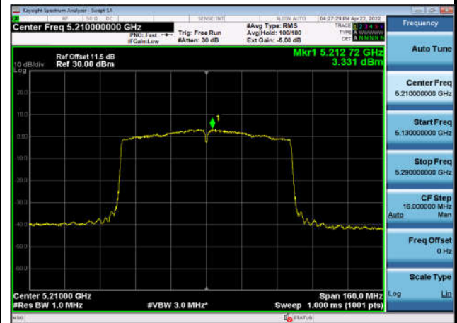
U-NII-1 Power spectral density-802.11 ax(20MHz),5220MHz,Ant1
