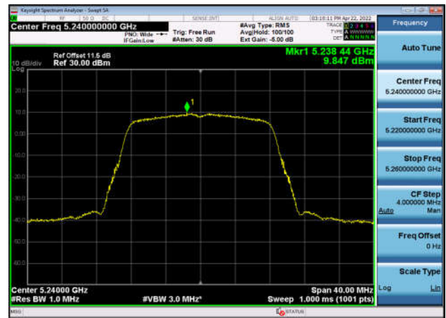
U-NII-1 Power spectral density-802.11 ac(20MHz),5220MHz,Ant1
