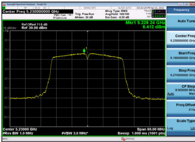
U-NII-1 Power spectral density-802.11 ax(20MHz),5180MHz,Ant1
