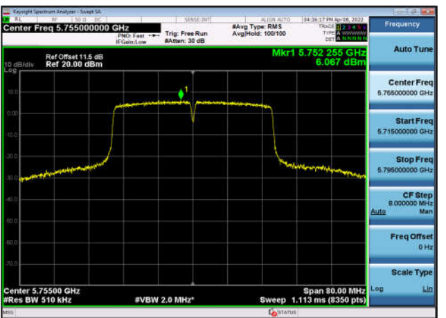
U-NII-3 Power spectral density-802.11 n(40MHz),5755MHz,Ant1
