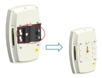
2. Fit the CPE on the wall, and mark the drilling locations.
