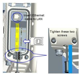
5. Connected Ethernet cable to the power adapter, as shown Figure 3-2.
