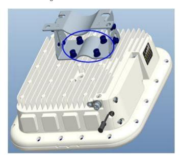
Figure 3-3 Install the Bracket
