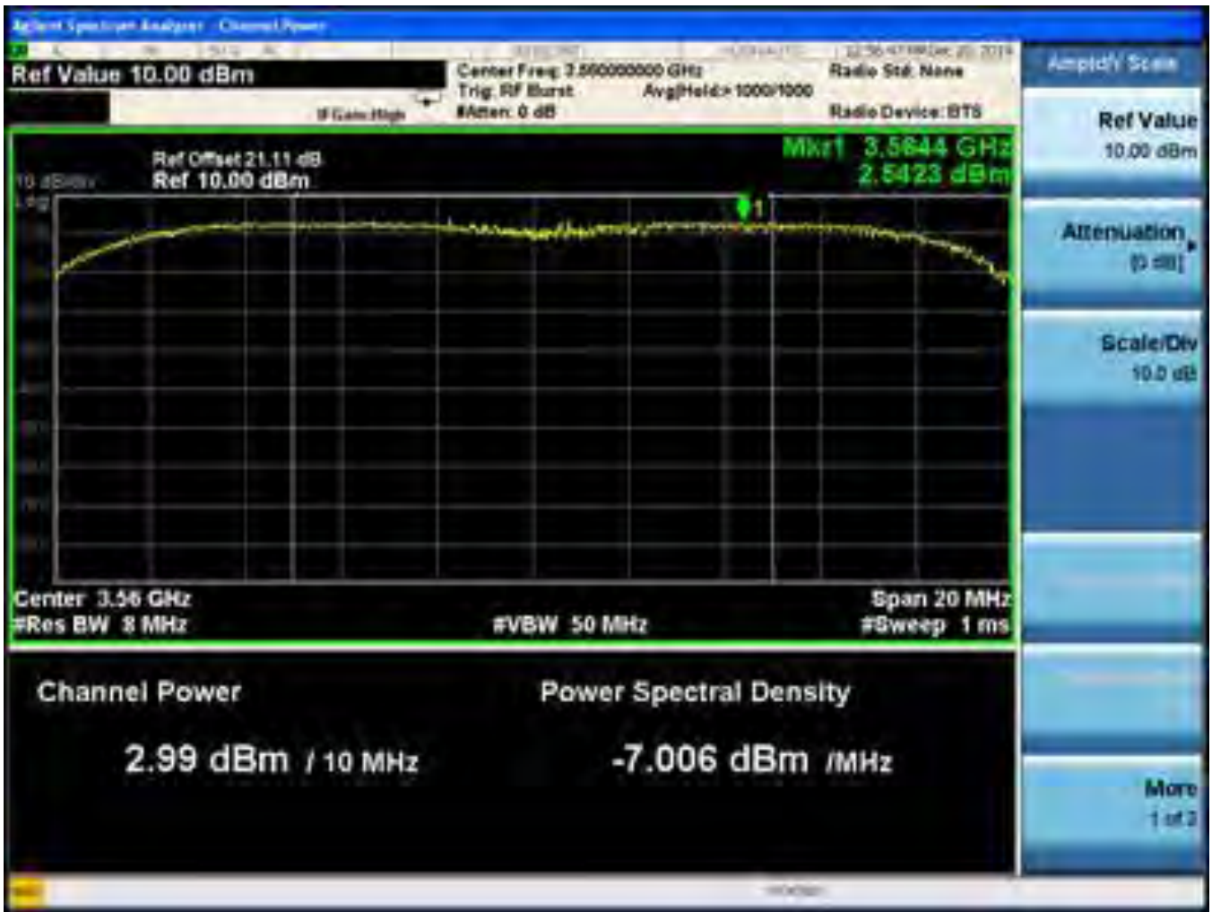
Figure CPE.KDB.2 A: MaxHold trace capture during registration and grant request procedure. This plot shows that the CPE-CBSD was able to register with test-SAS and obtain a grant operating at transmit power below 23dBm/10MHz EIRP.
