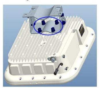
Figure 3-3 Install the Bracket
