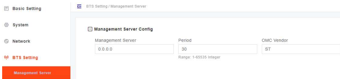
Figure 6-1 Configure Network Management Server
