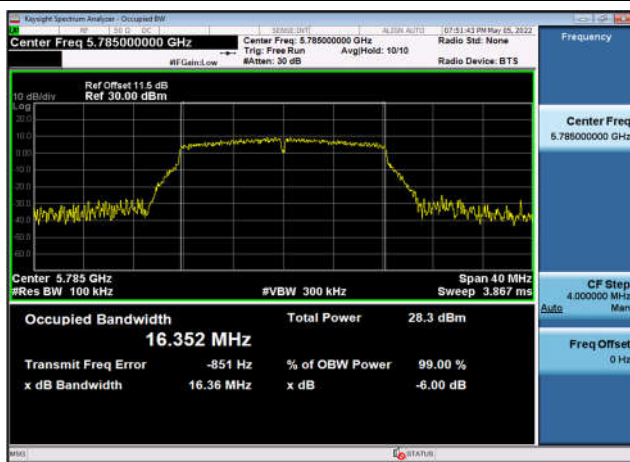
U-NII-3 6dB Bandwidth-802.11a(20MHz) ,5785MHz,Ant2
