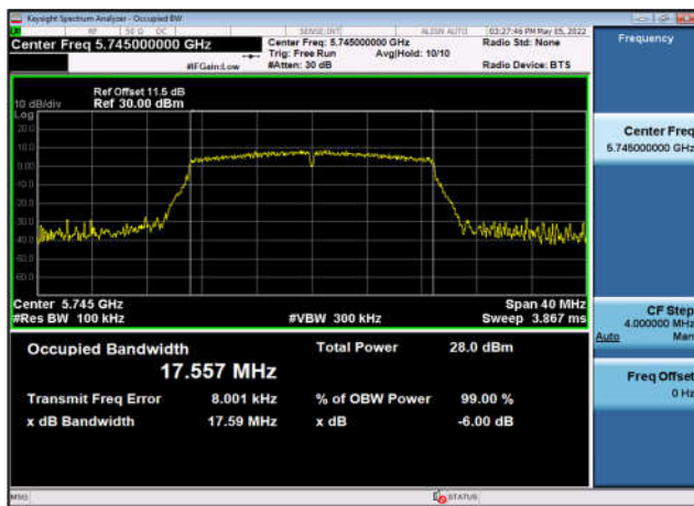
U-NII-3 6dB Bandwidth-802.11ac(20MHz) ,5745MHz,Ant1
