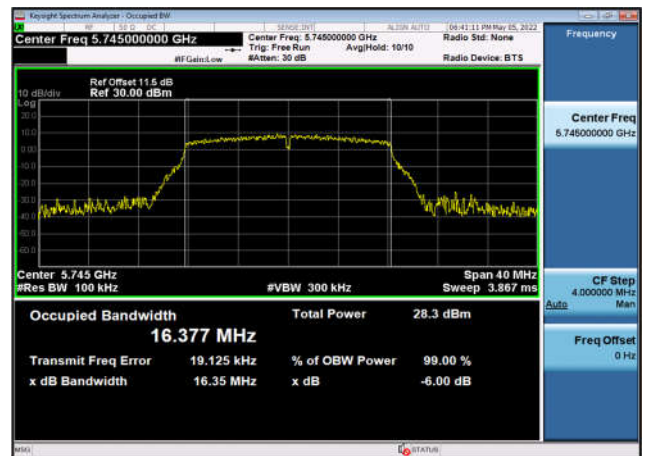
U-NII-3 6dB Bandwidth-802.11a(20MHz) ,5825MHz,Ant1
