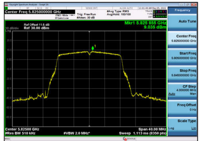
U-NII-3 Power spectral density-802.11 ac(20MHz),5785MHz,Ant0
