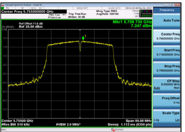
U-NII-3 Power spectral density-802.11 n(40MHz),5755MHz,Ant3
