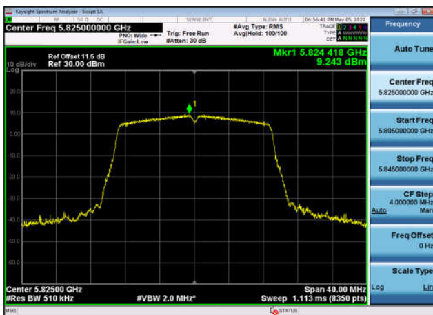
U-NII-3 Power spectral density-802.11 ac(20MHz),5825MHz,Ant2
