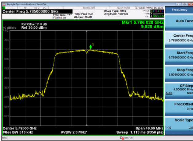
U-NII-3 Power spectral density-802.11 ac(20MHz),5745MHz,Ant2
