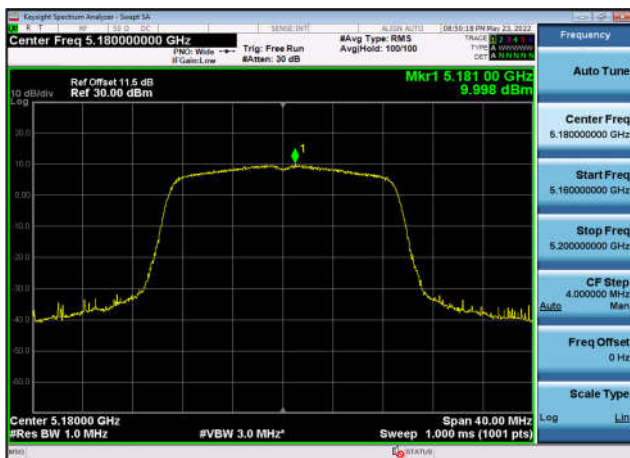
U-NII-1 Power spectral density-802.11 n(20MHz),5180MHz,Ant2
