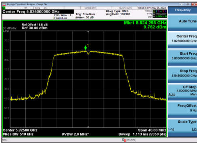
U-NII-3 Power spectral density-802.11 ax(40MHz),5795MHz,Ant0
