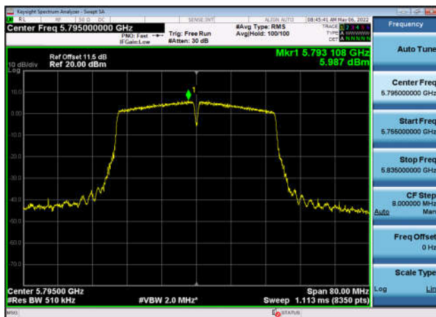
U-NII-3 Power spectral density-802.11 n(40MHz),5795MHz,Ant2
