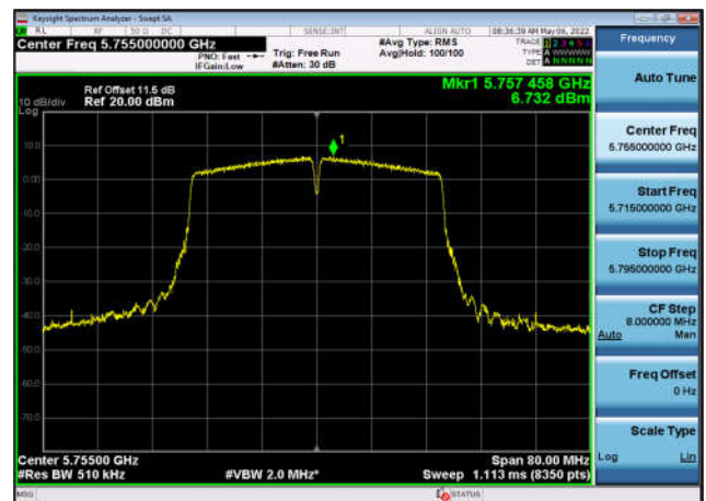
U-NII-3 Power spectral density-802.11 ac(40MHz),5755MHz,Ant2
