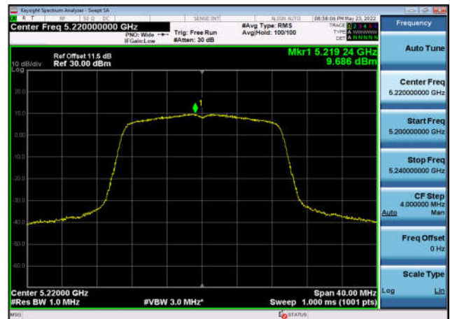
U-NII-1 Power spectral density-802.11 ac(20MHz),5220MHz,Ant1
