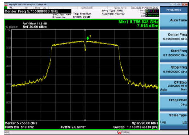
U-NII-3 Power spectral density-802.11 ax(80MHz),5775MHz,Ant1
