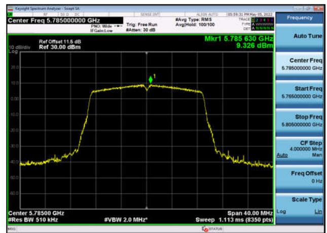
U-NII-3 Power spectral density-802.11 n(20MHz),5785MHz,Ant1
