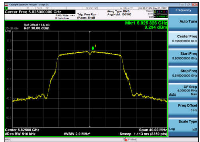
U-NII-3 Power spectral density-802.11 a(20MHz),5825MHz,Ant1
