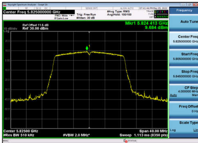
U-NII-3 Power spectral density-802.11 n(40MHz),5795MHz,Ant2
