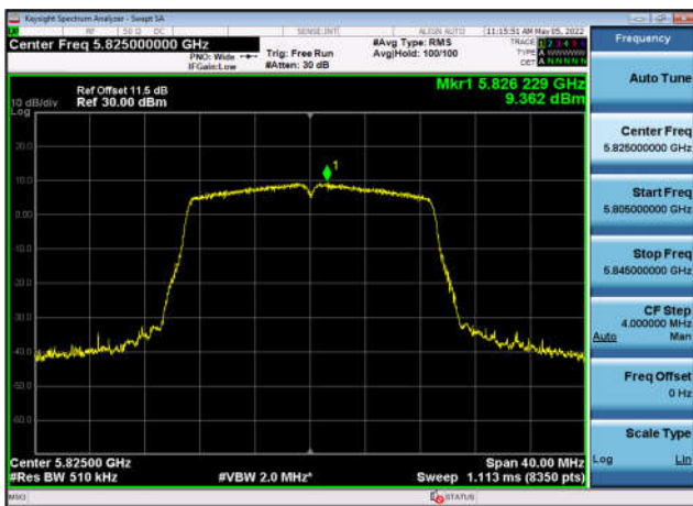
U-NII-3 Power spectral density-802.11 n(20MHz),5825MHz,Ant0
