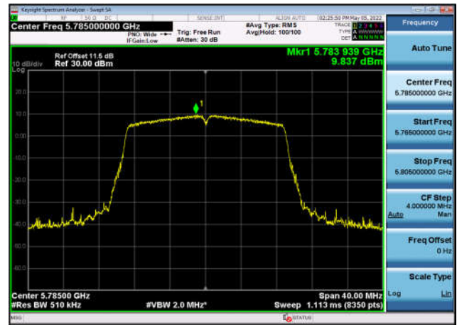
U-NII-3 Power spectral density-802.11 ax(40MHz),5755MHz,Ant1
