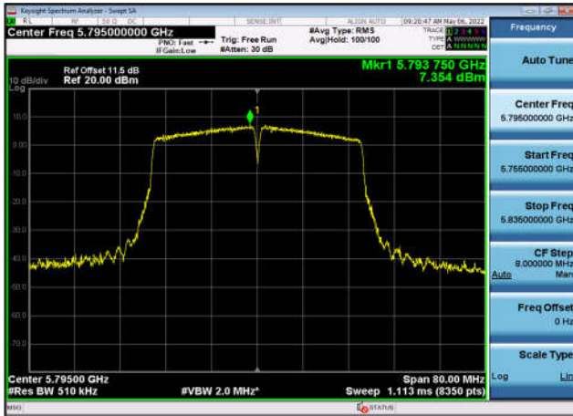
U-NII-3 Power spectral density-802.11 a(20MHz),5785MHz,Ant1
