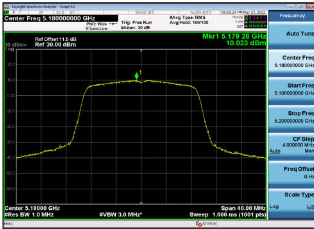
U-NII-1 Power spectral density-802.11 ac(20MHz),5240MHz,Ant2
