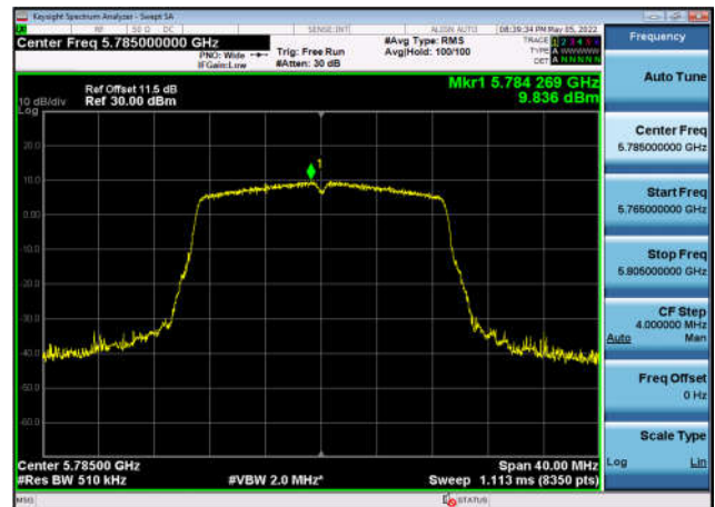
U-NII-3 Power spectral density-802.11 ac(20MHz),5785MHz,Ant3
