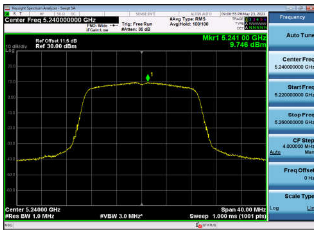
U-NII-1 Power spectral density-802.11 ax(20MHz),5240MHz,Ant3
