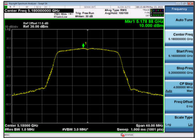
U-NII-1 Power spectral density-802.11 a(20MHz),5240MHz,Ant1
