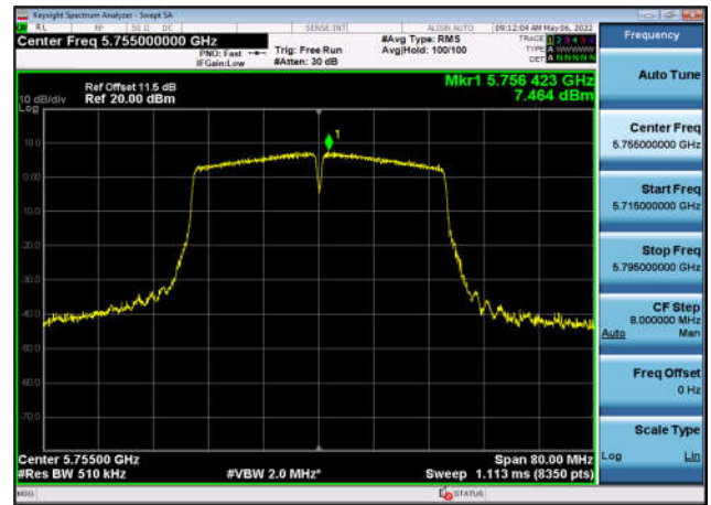
U-NII-3 Power spectral density-802.11 a(20MHz),5745MHz,Ant1
