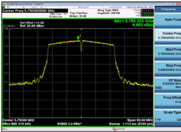
U-NII-3 Power spectral density-802.11 ax(20MHz),5745MHz,Ant2
