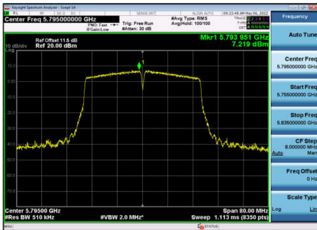
U-NII-3 Power spectral density-802.11 ax(20MHz),5745MHz,Ant3
