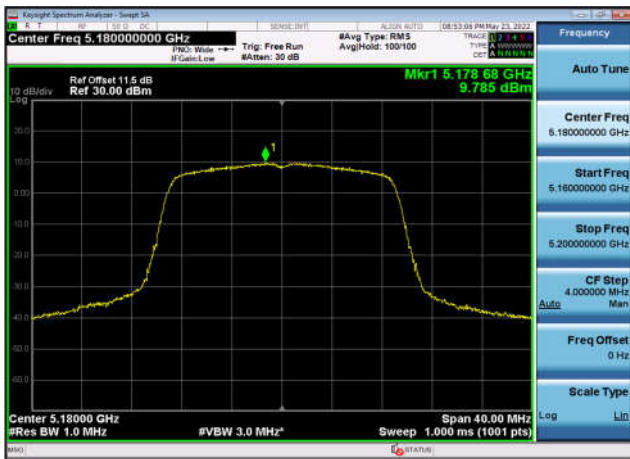
U-NII-1 Power spectral density-802.11 ac(20MHz),5240MHz,Ant0
