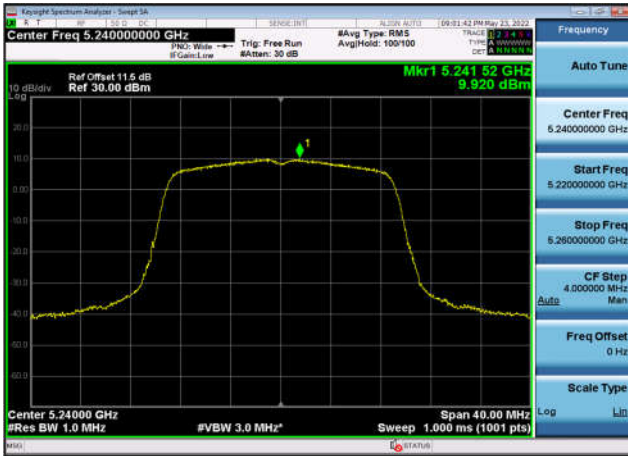
U-NII-1 Power spectral density-802.11 ac(40MHz),5230MHz,Ant1
