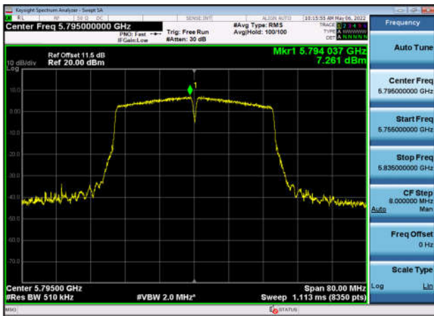
U-NII-3 Power spectral density-802.11 n(20MHz),5745MHz,Ant1
