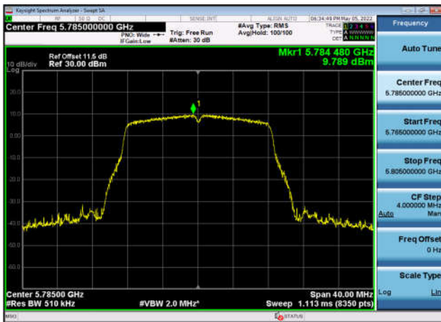
U-NII-3 Power spectral density-802.11 a(20MHz),5785MHz,Ant1
