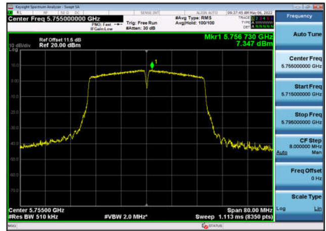
U-NII-3 Power spectral density-802.11 ac(80MHz),5775MHz,Ant3
