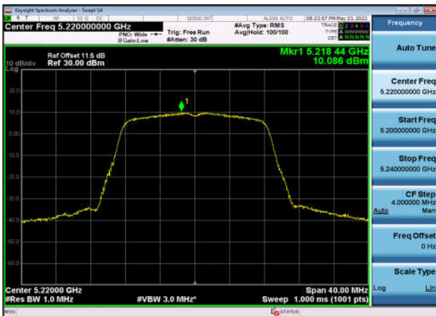
U-NII-1 Power spectral density-802.11 a(20MHz),5220MHz,Ant2
