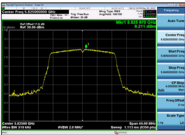
U-NII-3 Power spectral density-802.11 n(20MHz),5825MHz,Ant3
