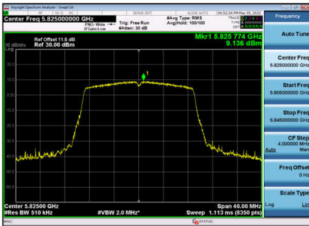
U-NII-3 Power spectral density-802.11 ac(40MHz),5795MHz,Ant1
