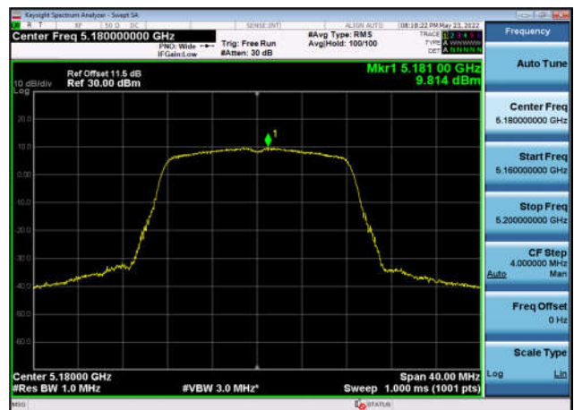
U-NII-1 Power spectral density-802.11 a(20MHz),5180MHz,Ant3
