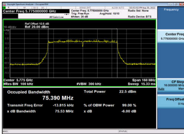
U-NII-3 6dB Bandwidth-802.11ax(20MHz) ,5745MHz,Ant0
