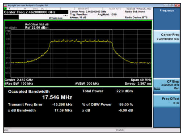
6dB Bandwidth-802.11n(HT20),2462MHz ,Ant1
