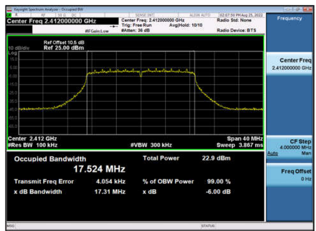
6dB Bandwidth-802.11n(HT20),2437MHz ,Ant1
