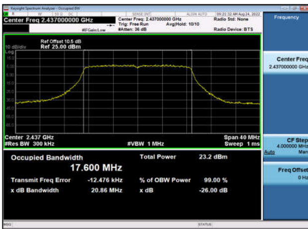
99% Bandwidth-802.11n(HT20),2462MHz ,Ant0
