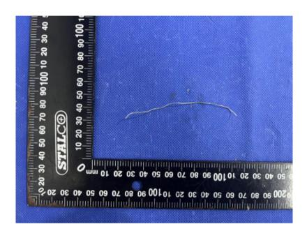
Remote control antenna specification Antenna size: 433M, antenna, material: Copper The antenna is whip with a width of 0.8mm a thickness of 1 oz and a total straightening length of 35mm Antenna Gain: OdBi
