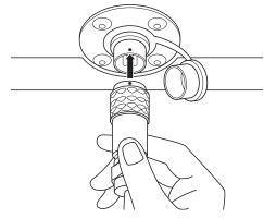
**5**. Gently push the plug into the input until the plug clicks into position.
