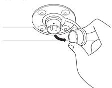
Align the red dot of the AC/DC Switching Adaptor with the red dot on the AC/DC Plug Input on the Sex Machine.
