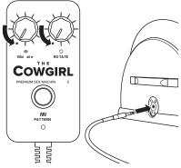
**3**. Gently push the **Corded Remote Control** plug into the remote control port on the **Sex Machine**.
