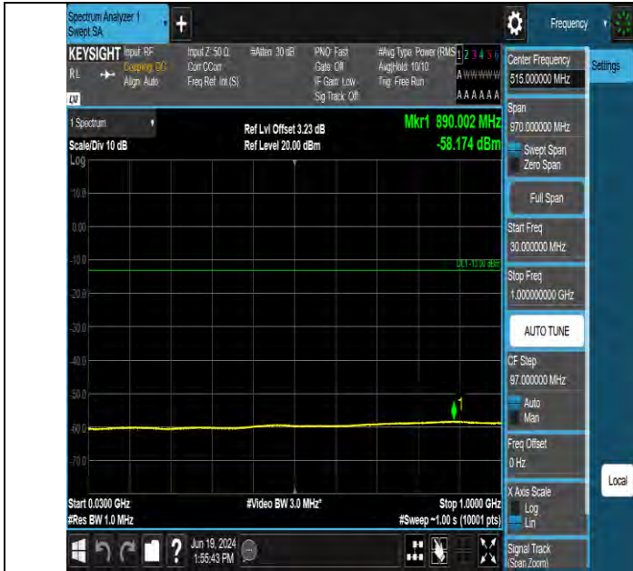
Band66 15MHz QPSK 132047 1RB#0 30~1000 30~1000
