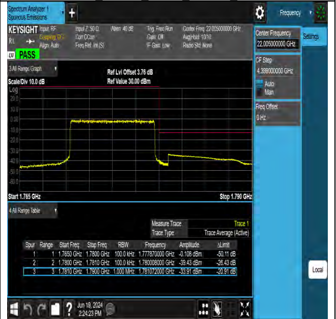
Band66 10MHz QPSK 132622 50RB#0
