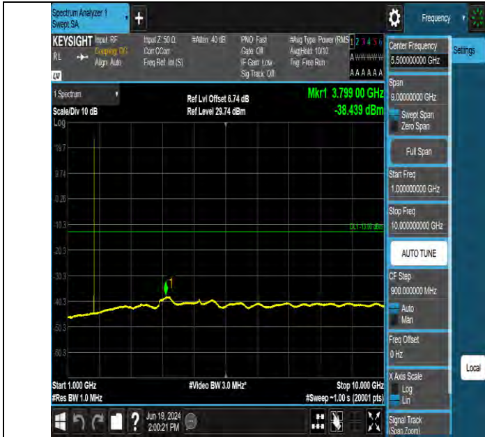
Band66 1.4MHz QPSK 132322 1RB#0 1000~10000 1000~10000
