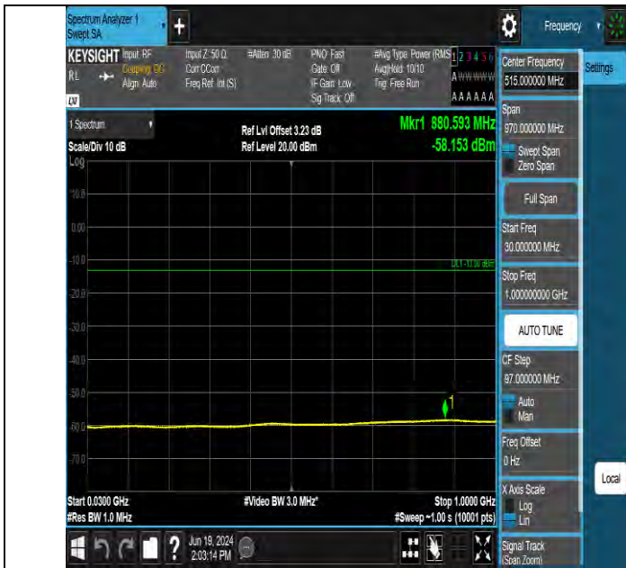
Band66 3MHz QPSK 132322 1RB#0 30~1000 30~1000
