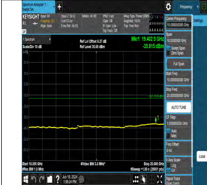
Band66 15MHz QPSK 132047 1RB#0 10000~20000 10000~20000
