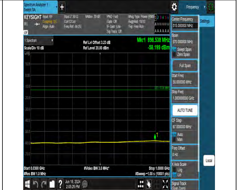
Band66 10MHz QPSK 132022 1RB#0 30~1000 30~1000
