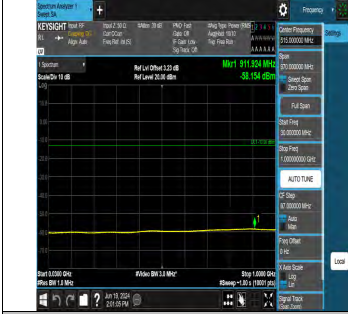
Band66 1.4MHz QPSK 132665 1RB#0 30~1000 30~1000
