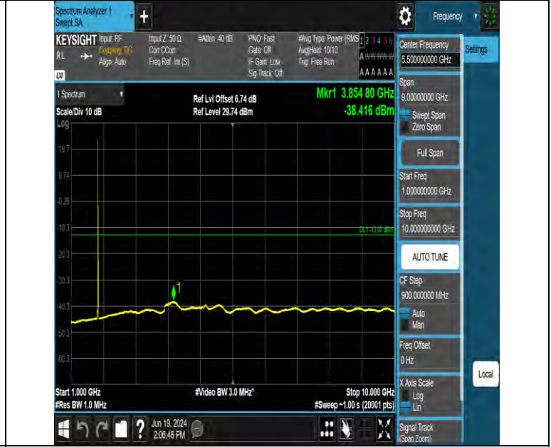
Band66 10MHz QPSK 132322 1RB#0 1000~10000 1000~10000
