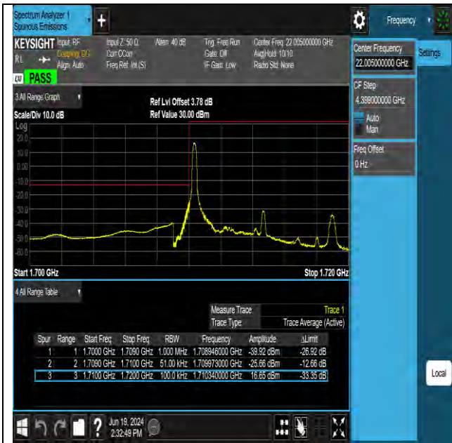
Band66 5MHz 16QAM 131997 1RB#0
