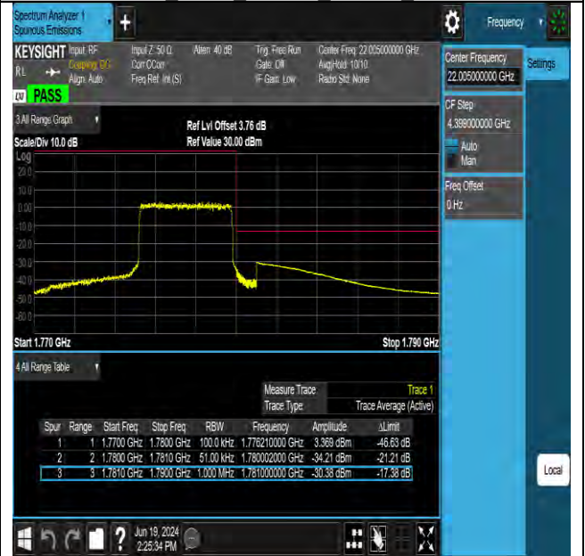
Band66 5MHz 16QAM 132647 25RB#0
