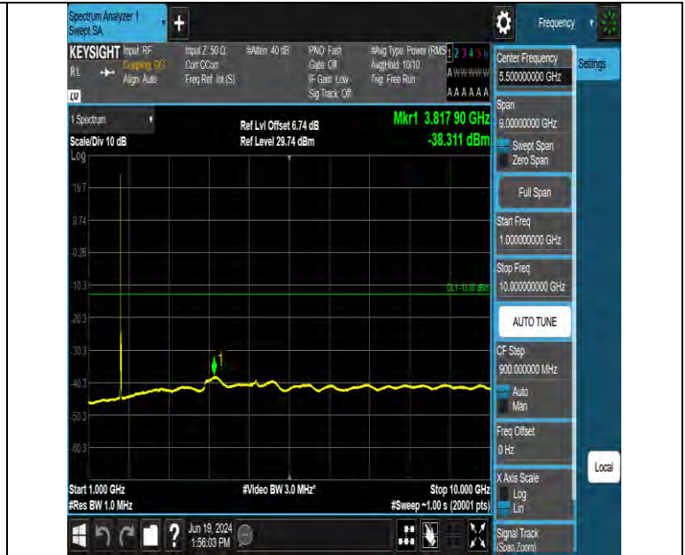
Band66 15MHz QPSK 132047 1RB#0 1000~10000 1000~10000
