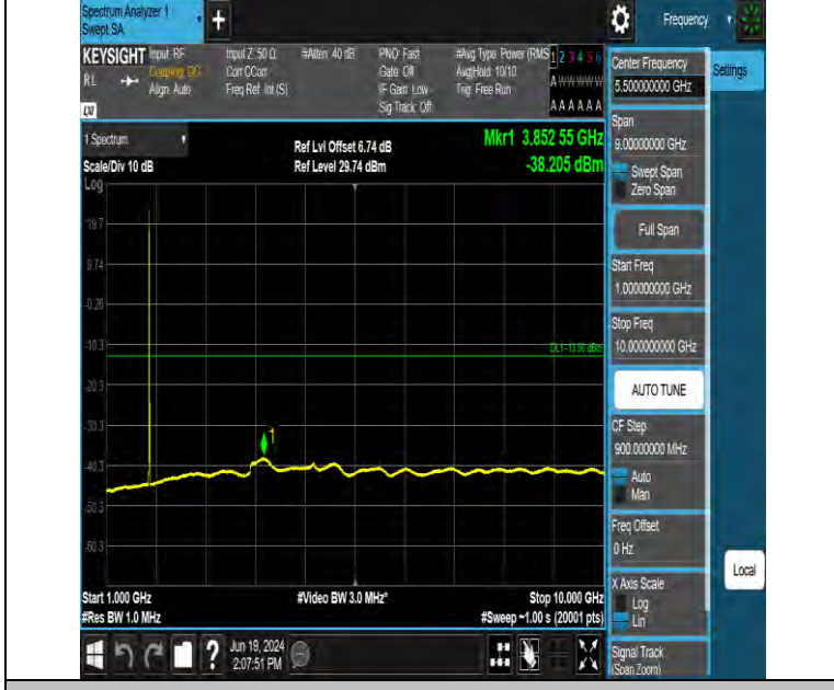
Band66 10MHz QPSK 132622 1RB#0 1000~10000 1000~10000
