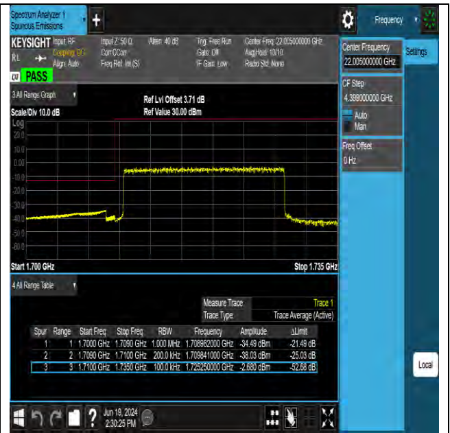
Band66 20MHz 16QAM 132072 100RB#0
