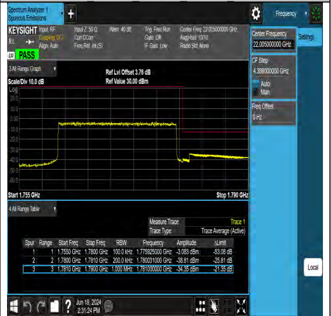
Band66 20MHz 16QAM 132572 100RB#0
