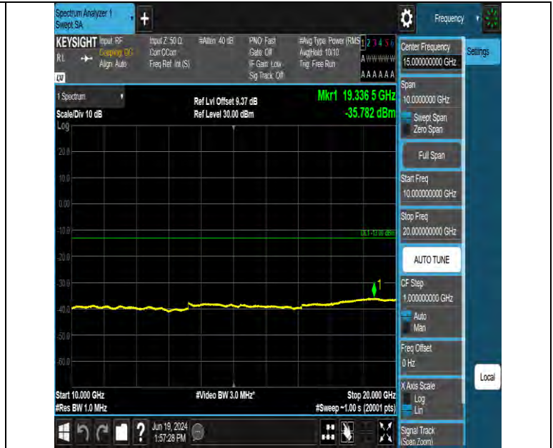
Band66 15MHz QPSK 132322 1RB#0 10000~20000 10000~20000
