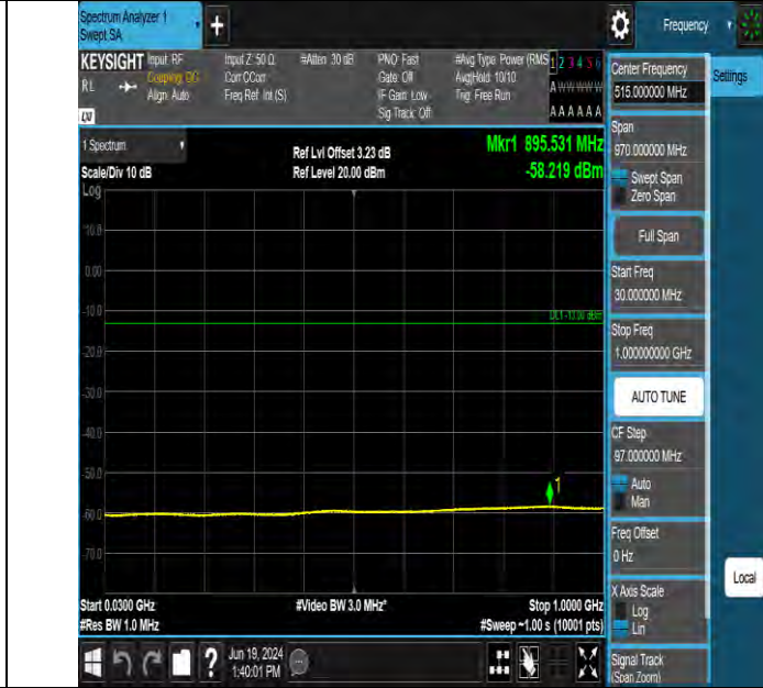
Band2 10MHz QPSK 18900 1RB#49 30~1000 30~1000
