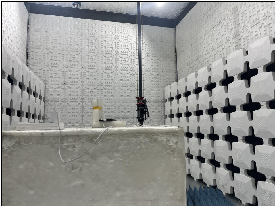
Radiated emission test: Frequency Range < Above 1GHz >
