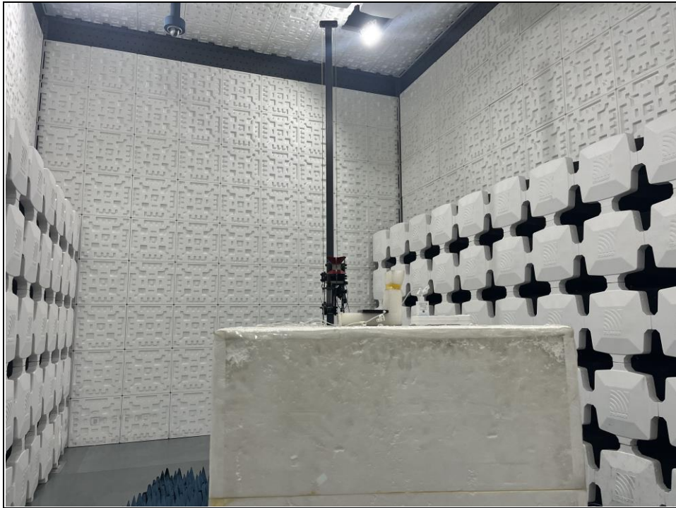
Radiated emission test: Frequency Range < 9KHz- 30MHz >
