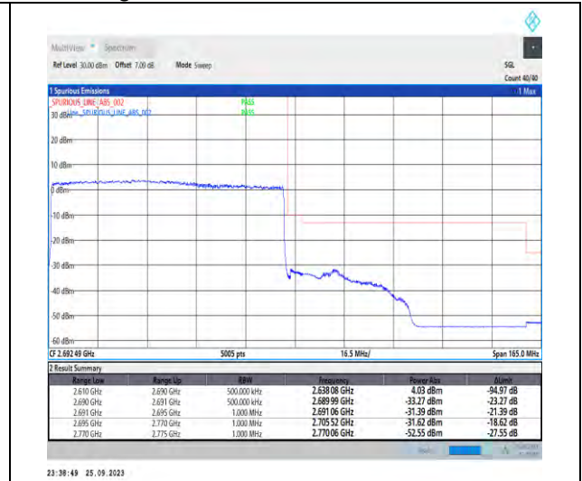
1-N41-PC3-30-80-H-3-DFT-PI2BPSK-Outer_Full-2 16@0-Ant5-1--PASS-see graph
