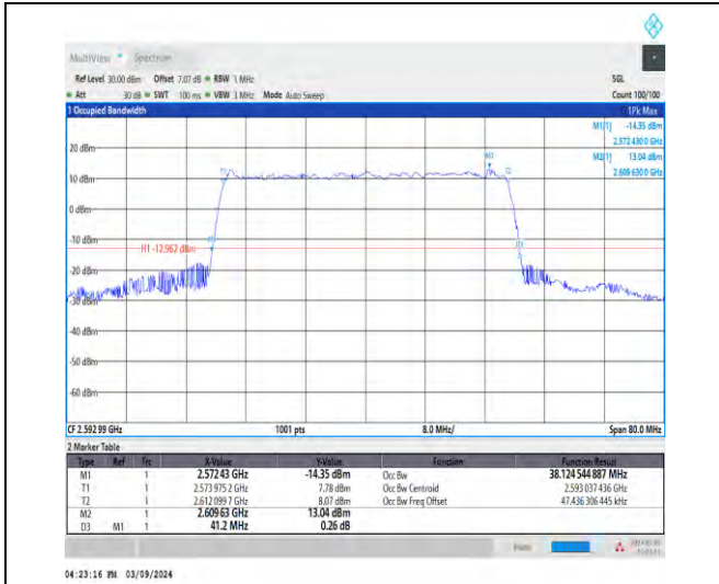
1-N41-30-40-M-9-CP-256QAM-Outer_Full-106@0-A nt1-38.125-41.200-≤40-PASS
