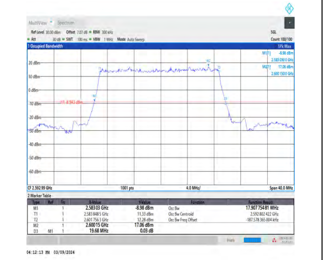
1-N41-30-20-M-2-DFT-PI2BPSK-Outer_Full-50@0-Ant1 -17.908-19.680-≤20-PASS
