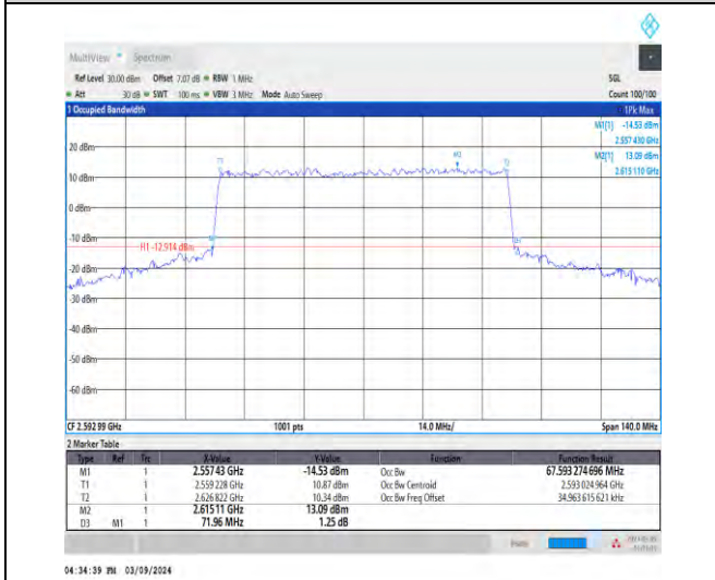
1-N41-30-70-M-8-CP-64QAM-Outer_Full-189@0-Ant1 t1-67.593-71.960-≤70-PASS
