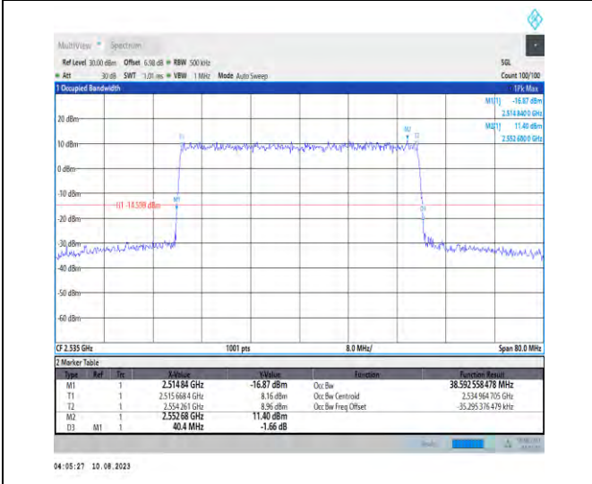
1-N7-PC3-15-40-M-5-DFT-256QAM-Outer_Full-216 @0-Ant1-38.593-40.400-≤40-PASS
