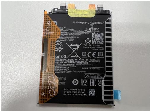
Model Name: BM5V Rated capacity: 5020mAh
