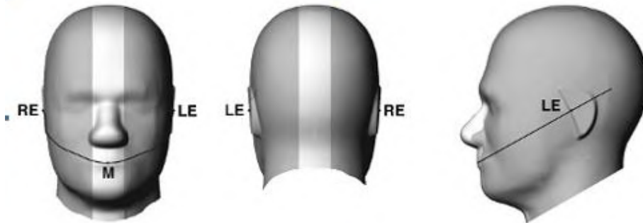
F-3. Front, back, and side views of SAM (model for the phantom shell). Full-head model is for illustration purposes only-procedures in this recommended practice are intended primarily for the phantom setup.
