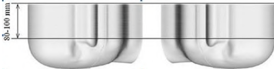
F-4. Sagittally bisected phantom with extended perimeter (shown placed on its side as used for SAR measurements)
