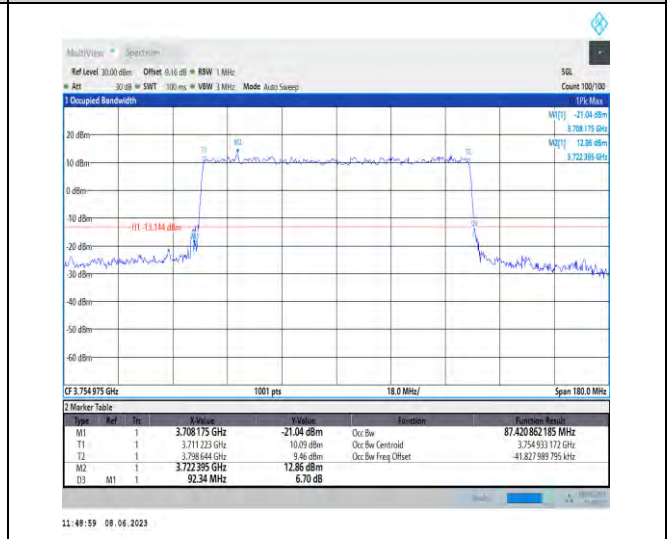
1-N78-3700-3800-PC3-30-90-H-8-CP-64QAM-Outer _Full-245@0-Ant1-87.421-92.340-≤90-PASS
