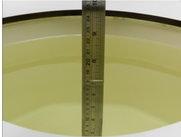
Fig 11.1 Photo of Liquid Height for Body SAR
