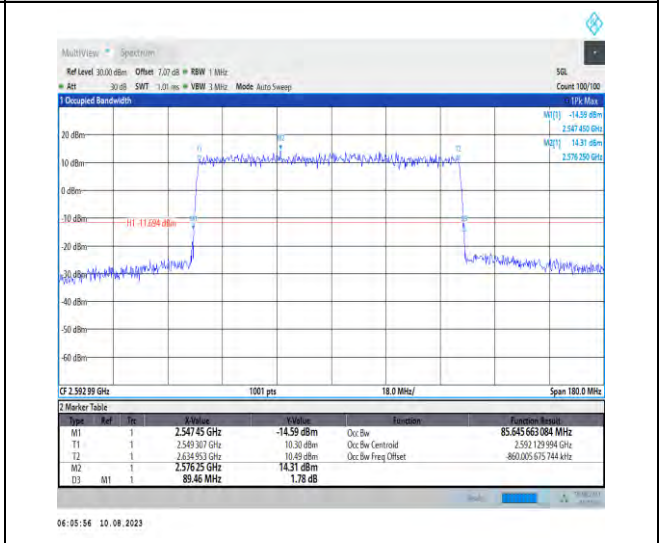
1-N41-PC3-30-90-M-1-DFT-QPSK-Outer_Full-240@ 0-Ant1-85.646-89.460-<90-PASS
