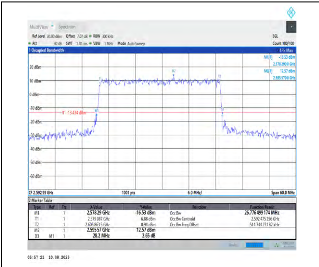
1-N41-PC3-30-30-M-4-DFT-64QAM-Outer_Full-75@ 0-Ant1-26.776-28.200-≤30-PASS
