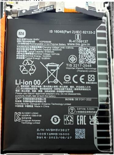
Model Name: BM5V Rated capacity: 5020mAh Brand Name:MI Manufacturer: Sunwoda
