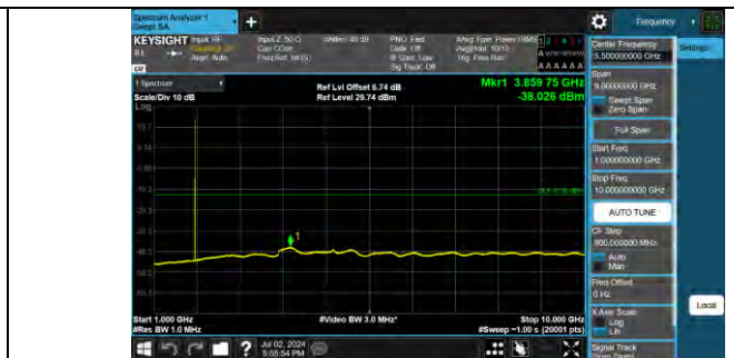
Band2 1.4MHz QPSK 18607 1RB#0 1000~10000 1000~10000
