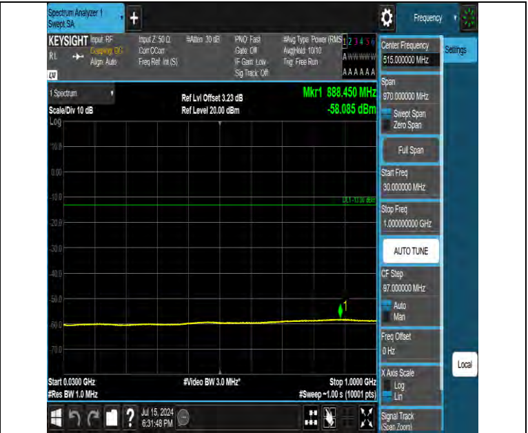
Band66 10MHz QPSK 132622 1RB#0 30~1000 30~1000
