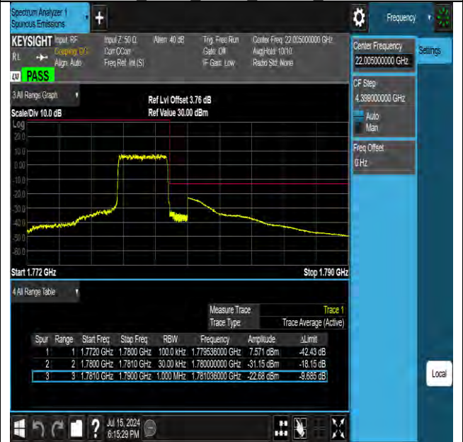
Band66 3MHz QPSK 132657 15RB#0
