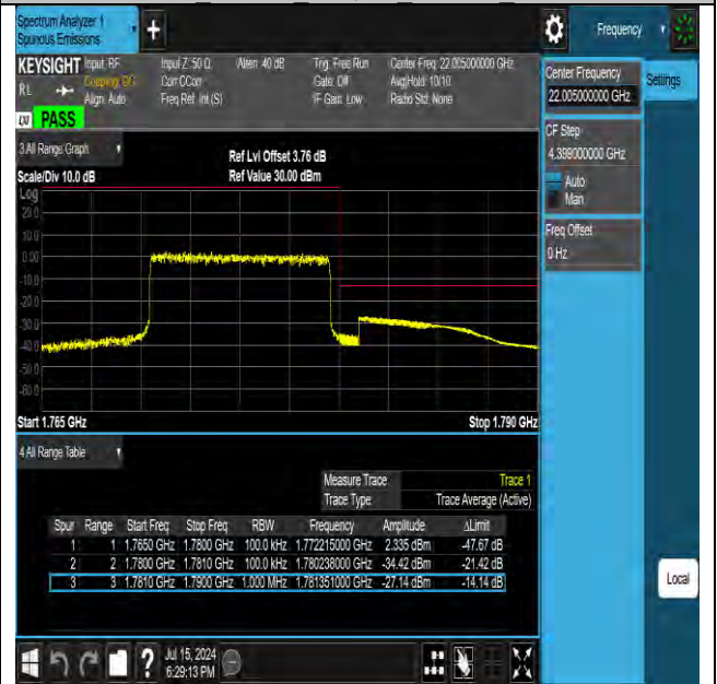
Band66 10MHz 16QAM 132622 50RB#0
