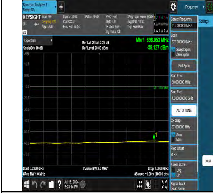
Band66 5MHz QPSK 131997 1RB#0 30~1000 30~1000
