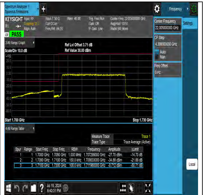
Band66 15MHz 16QAM 132047 75RB#0
