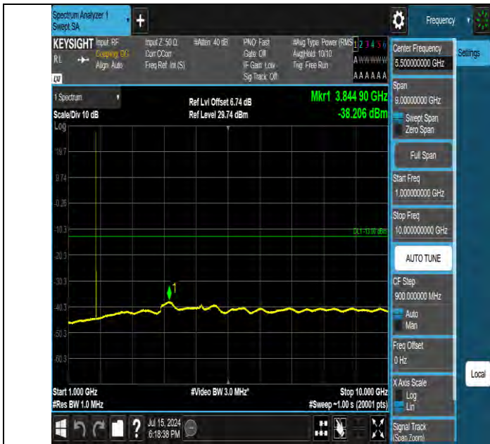
Band66 3MHz QPSK 132657 1RB#0 1000~10000 1000~10000
