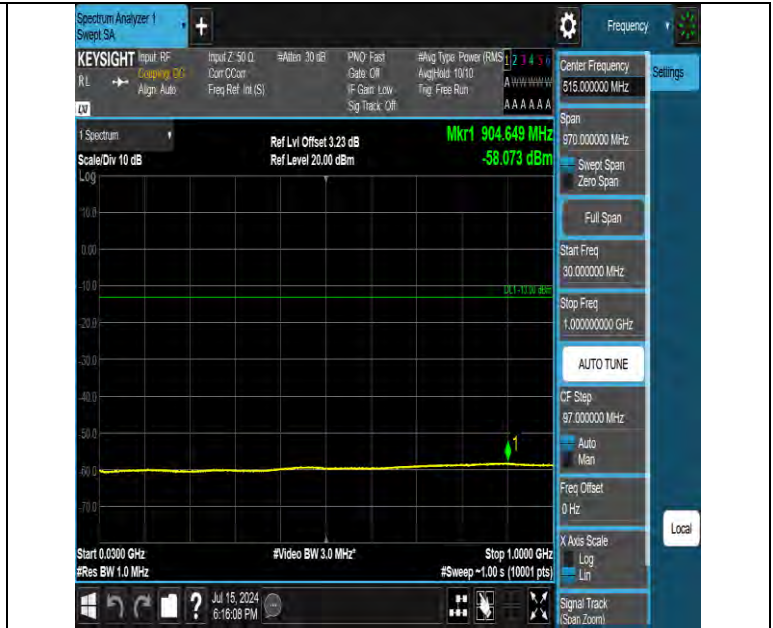
Band66 3MHz QPSK 131987 1RB#0 30~1000 30~1000
