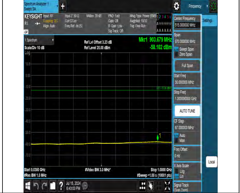
Band66 15MHz QPSK 132322 1RB#0 30~1000 30~1000
