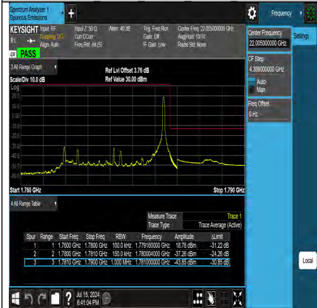
Band66 15MHz 16QAM 132597 1RB#74
