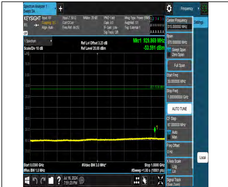
Band42 20MHz QPSK 42590 1RB#0 30~1000 30~1000
