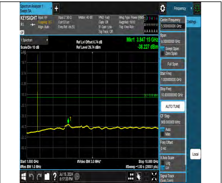
Band66 3MHz QPSK 132322 1RB#0 1000~10000 1000~10000
