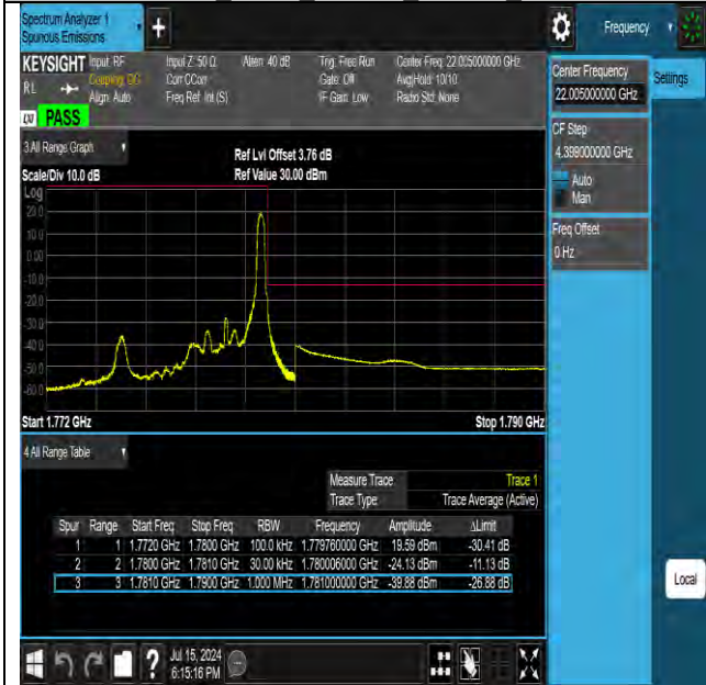
Band66 3MHz 16QAM 132657 1RB#14
