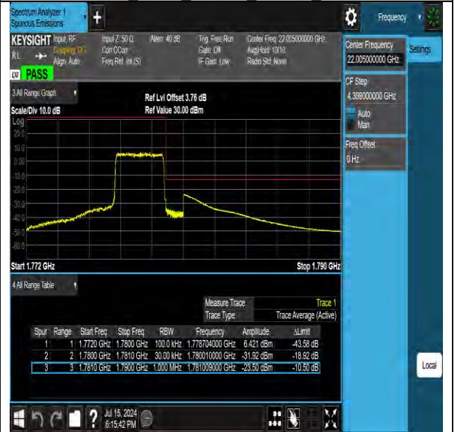
Band66 3MHz 16QAM 132657 15RB#0
