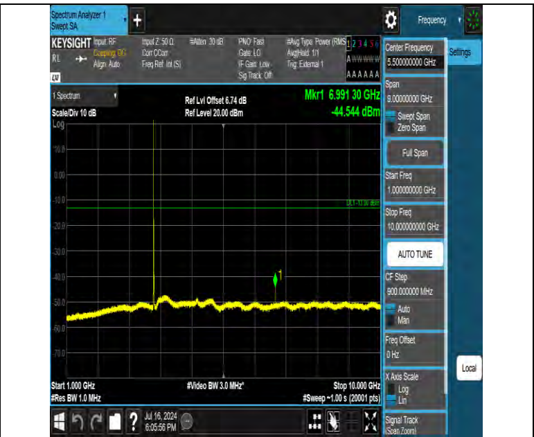
Band42 10MHz QPSK 42590 1RB#0 1000~10000 1000~10000
