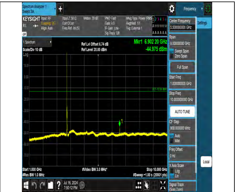
Band42 20MHz QPSK 42190 1RB#0 1000~10000 1000~10000
