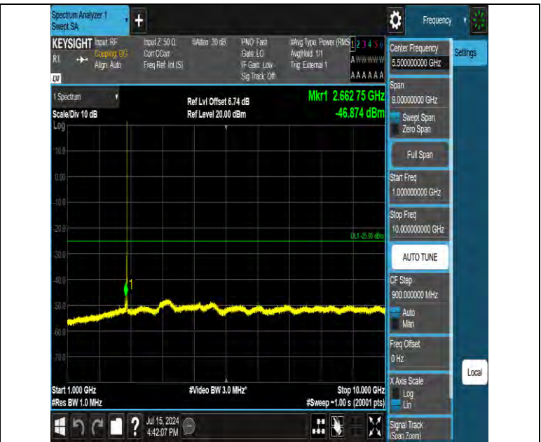
Band41 5MHz QPSK 41565 1RB#0 1000~10000 1000~10000
