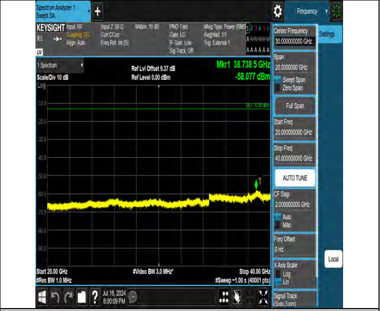
Band42 5MHz QPSK 43065 1RB#0 20000~40000 20000~40000
