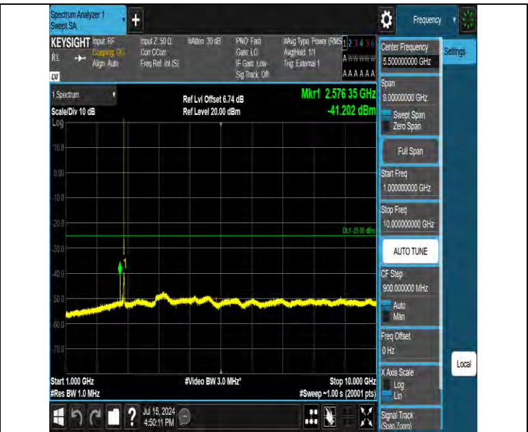
Band41 10MHz QPSK 41540 1RB#0 1000~10000 1000~10000
