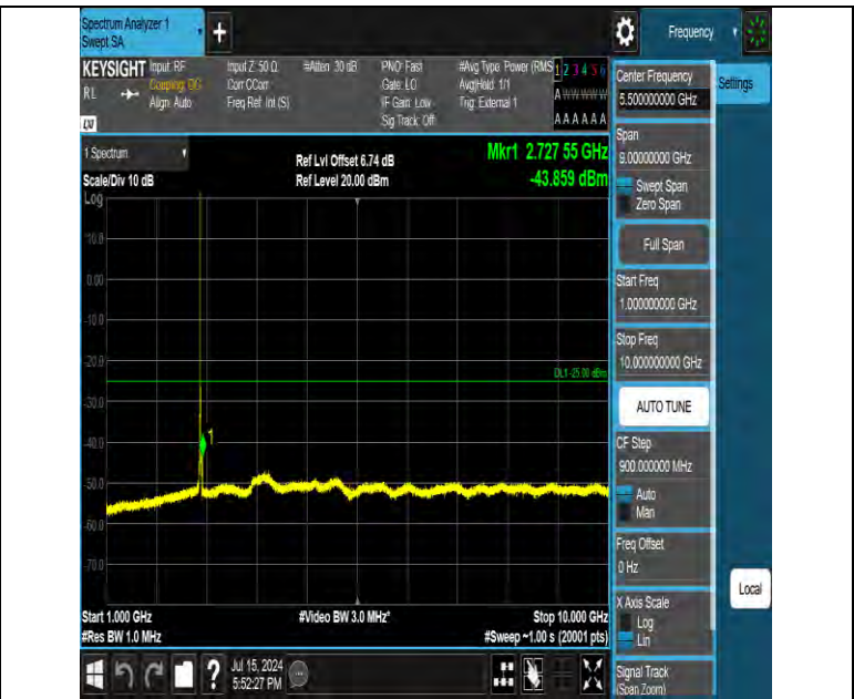
Band41 15MHz QPSK 41515 1RB#0 1000~10000 1000~10000
