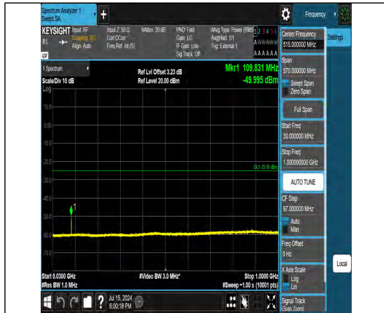
Band41 20MHz QPSK 41490 1RB#0 30~1000 30~1000
