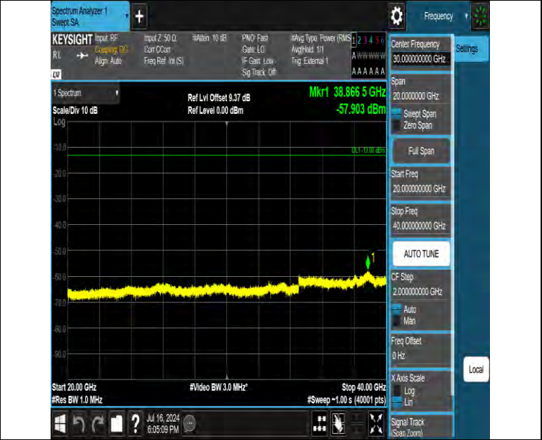
Band42 10MHz QPSK 42140 1RB#0 20000~40000 20000~40000
