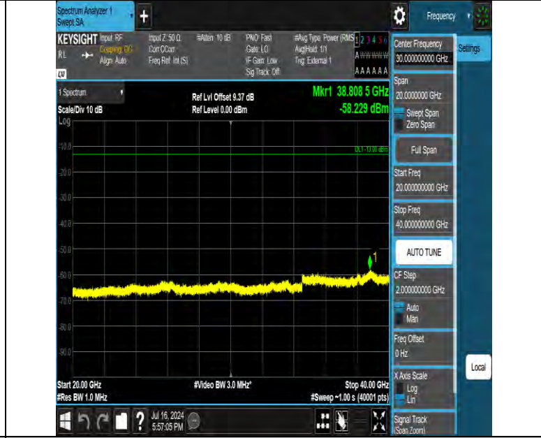
Band42 5MHz QPSK 42115 1RB#0 20000~40000 20000~40000
