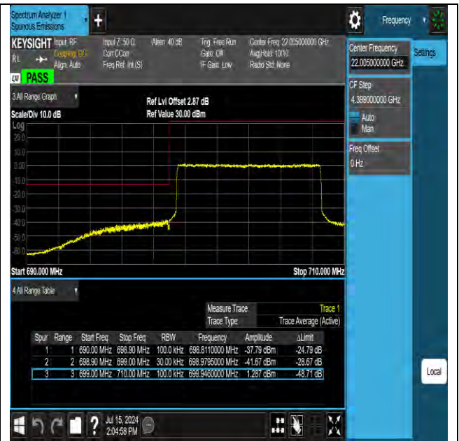
Band12 10MHz 16QAM 23060 50RB#0
