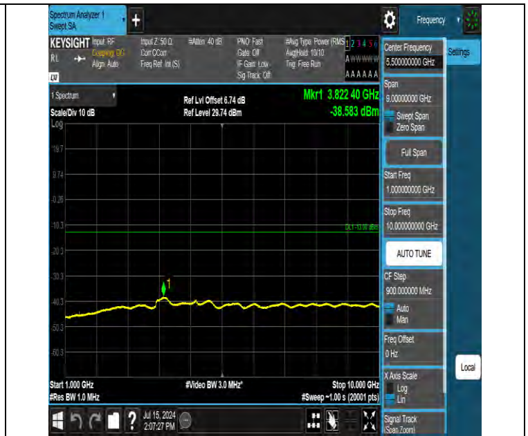
Band12 10MHz QPSK 23095 1RB#0 1000~10000 1000~10000
