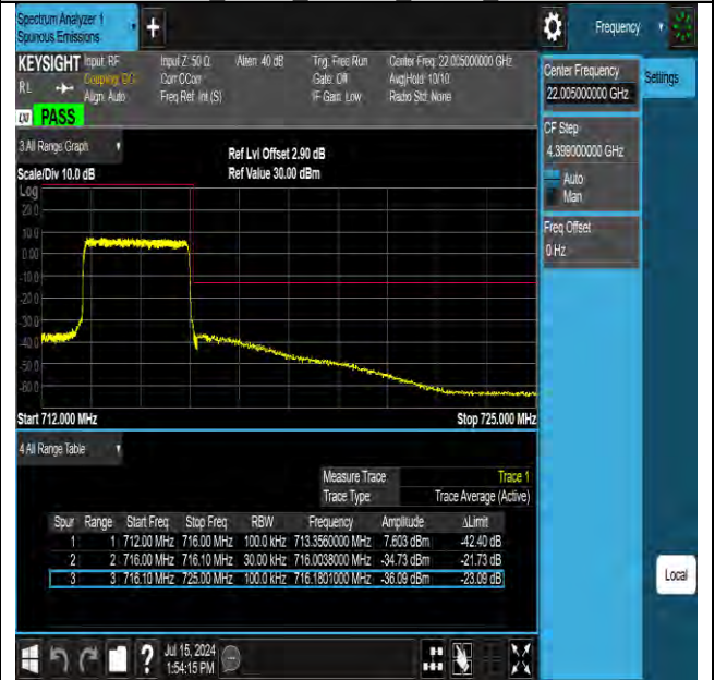
Band12 3MHz 16QAM 23165 15RB#0
