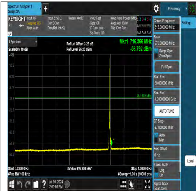
Band12 5MHz QPSK 23035 1RB#0 30~1000 30~1000
