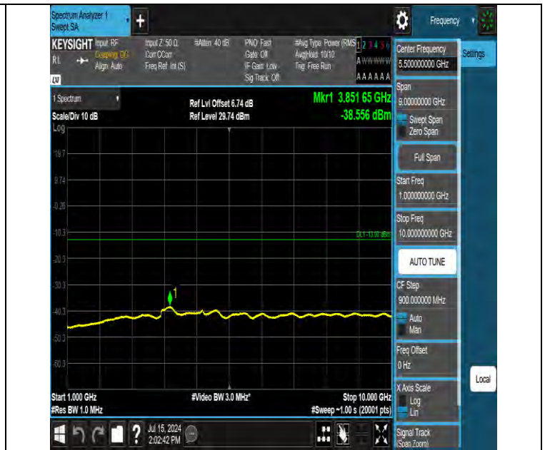
Band12 5MHz QPSK 23155 1RB#0 1000~10000 1000~10000
