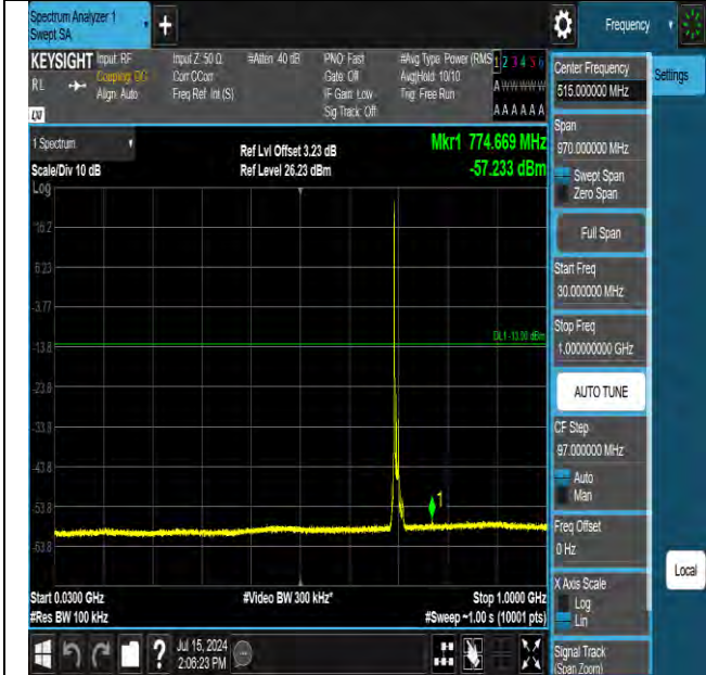
Band12 10MHz QPSK 23060 1RB#0 30~1000 30~1000
