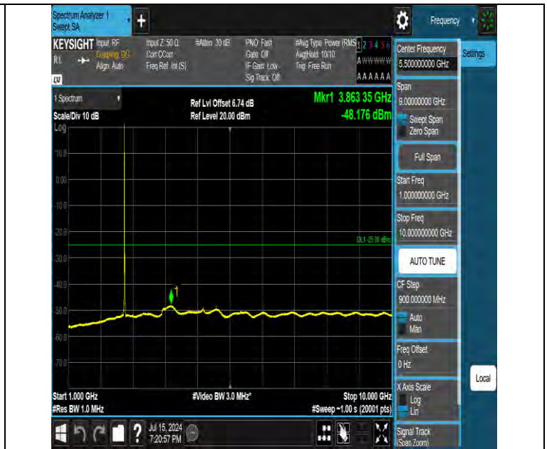
Band7 15MHz QPSK 21375 1RB#0 1000~10000 1000~10000
