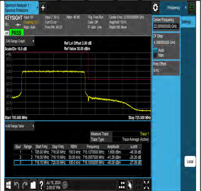
Band12 10MHz 16QAM 23130 50RB#0
