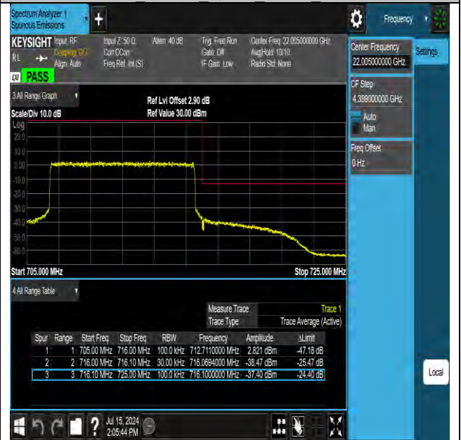
Band12 10MHz QPSK 23130 50RB#0
