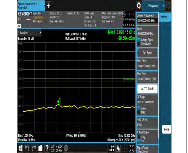
Band12 5MHz QPSK 23095 1RB#0 1000~10000 1000~10000
