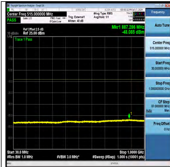
NTNV-N77-3450-3550-PC2-30-30-M-DFT-QPSK-Edge 1RB Left-Ant1-PASS
