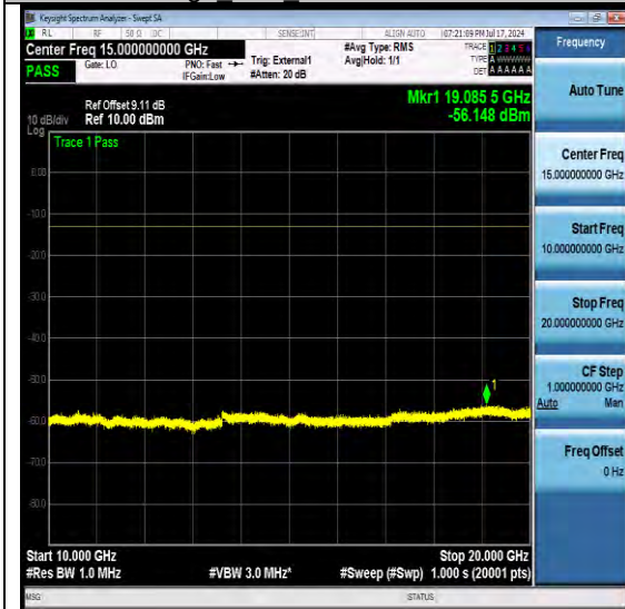
NTNV-N77-3700-3980-PC2-30-60-M-DFT-QPSK-Edge 1RB Left-Ant1-PASS
