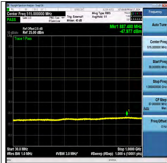
NTNV-N77-3700-3980-PC2-30-30-M-DFT-QPSK-Edge 1RB Left-Ant1-PASS
