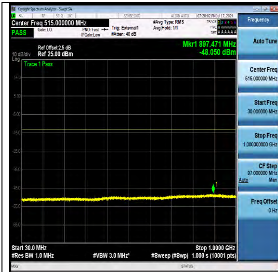
NTNV-N77-3700-3980-PC2-30-100-L-DFT-QPSK-Edge 1RB Left-Ant1-PASS
