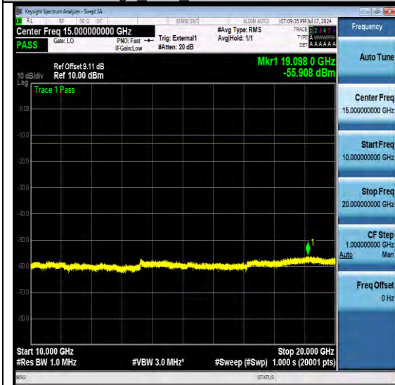
NTNV-N77-3700-3980-PC2-30-30-M-DFT-QPSK-Edge 1RB Left-Ant1-PASS
