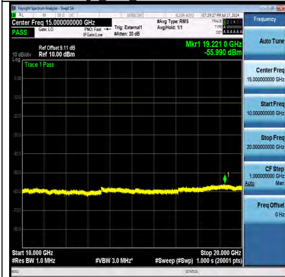
NTNV-N77-3700-3980-PC2-30-100-L-DFT-QPSK-Edge 1RB Left-Ant1-PASS
