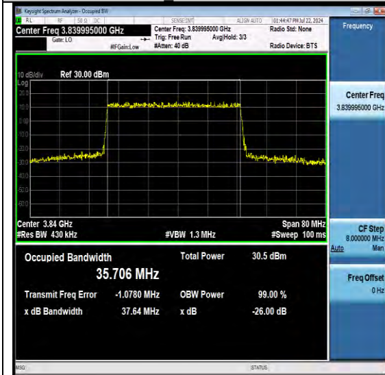
NTNV-N77-3700-3980-PC2-30-40-M-DFT-16QAM -Outer Full-Ant1-PASS
