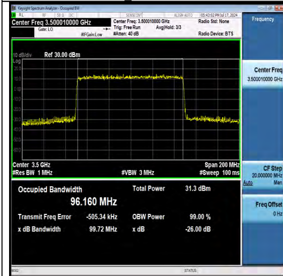
NTNV-N77-3450-3550-PC2-30-100-M-DFT-16QA M-Outer Full-Ant1-PASS
