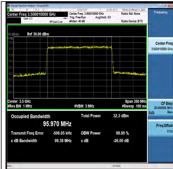
NTNV-N77-3450-3550-PC2-30-100-M-DFT-PI2BP SK-Outer Full-Ant1-PASS
