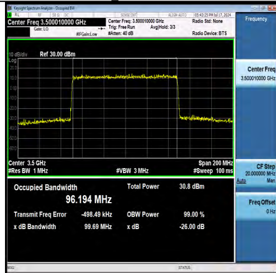
NTNV-N77-3450-3550-PC2-30-100-M-DFT-64QA M-Outer Full-Ant1-PASS
