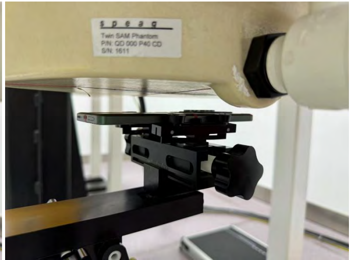
Rear Face of EUT with 2.0 cm Gap (Body-Worn Mode)
