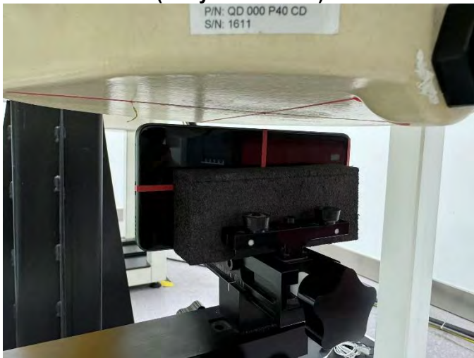
Left Side of EUT with 1 cm Gap (Body-Worn Mode)
