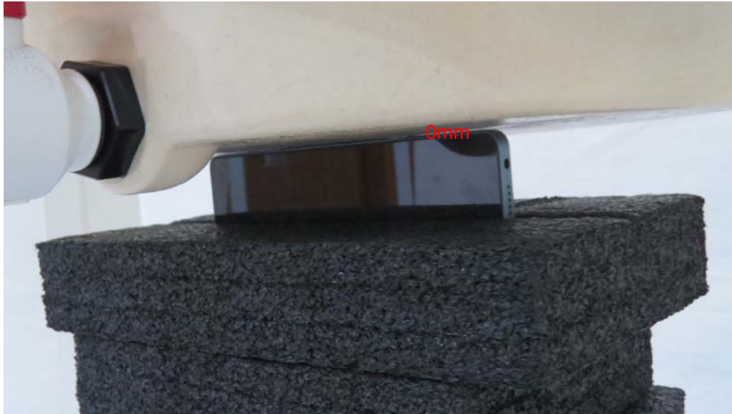
Picture 15: Left Edge, the distance from EUT to the bottom of the Phantom is 0mm
