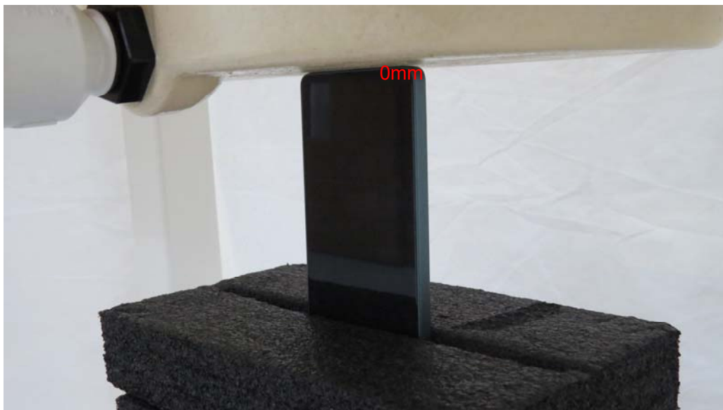
Picture 18: Bottom Edge, the distance from EUT to the bottom of the Phantom is 0mm
