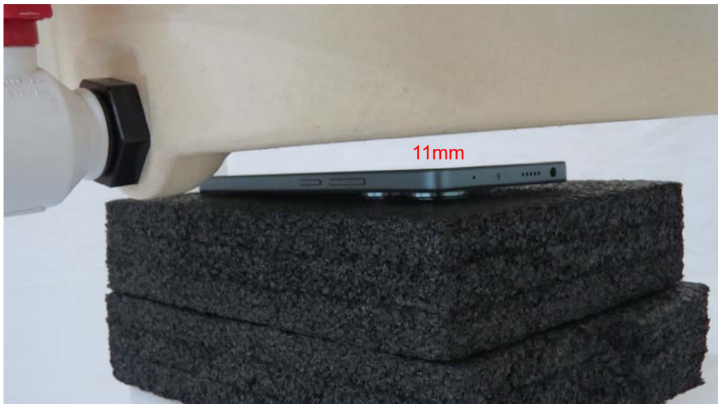
Picture 22: Front Side, the distance from EUT to the bottom of the Phantom is 11mm
