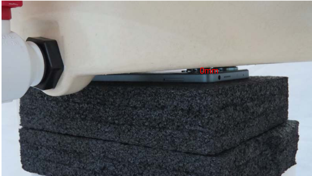
Picture 13: Back Side, the distance from EUT to the bottom of the Phantom is 0mm
