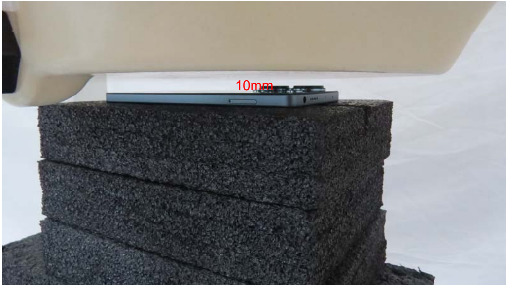
Picture 7: Back Side, the distance from EUT to the bottom of the Phantom is 10mm
