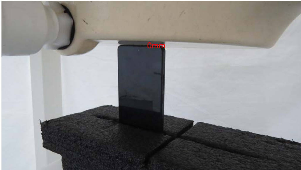
Picture 25: Top Edge, the distance from EUT to the bottom of the Phantom is 0mm
