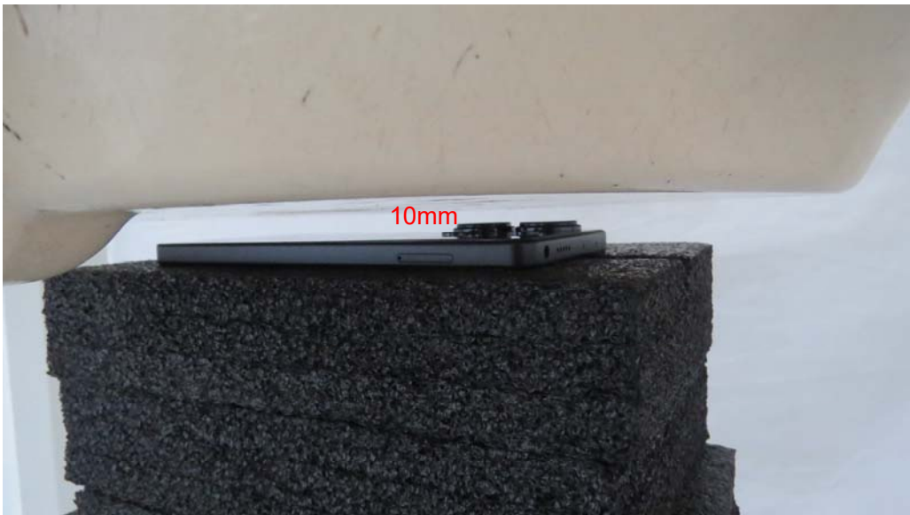
Picture 24: Back Side, the distance from EUT to the bottom of the Phantom is 10mm
