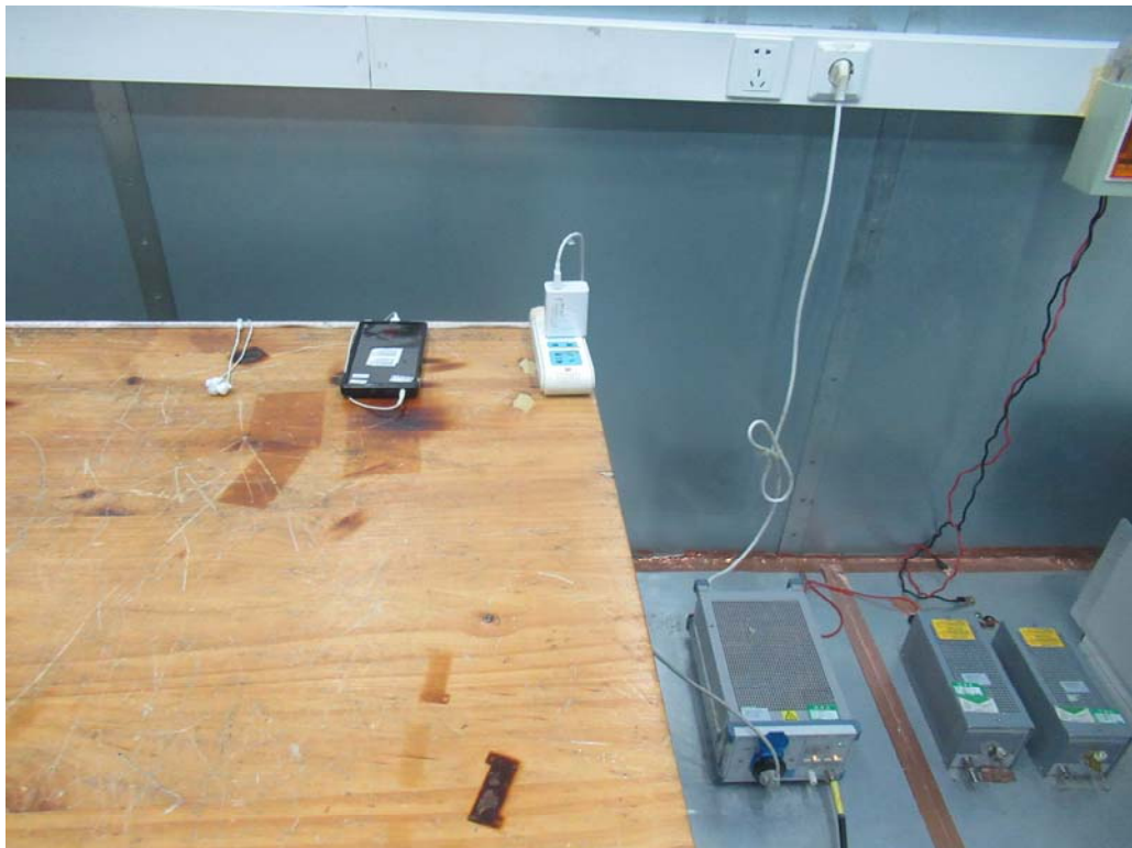
Picture 2 Conducted Emission Test Setup
