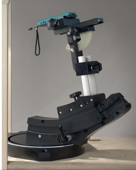
F-2. Device Holder for Transmitters
