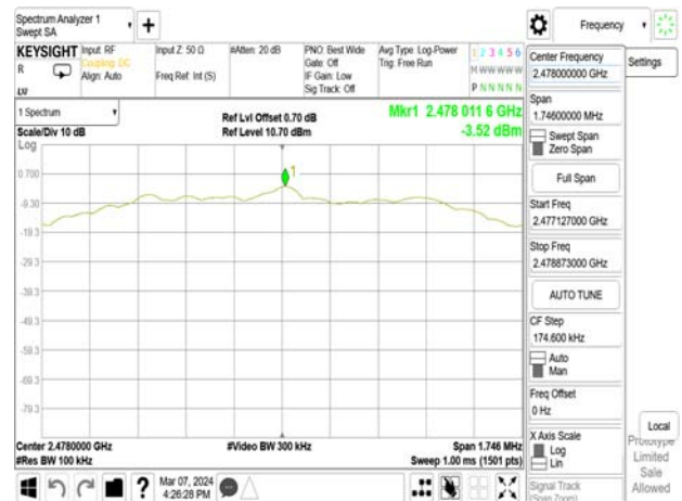
Reference Level_BLE 2M_HighCH38-2478MHz
