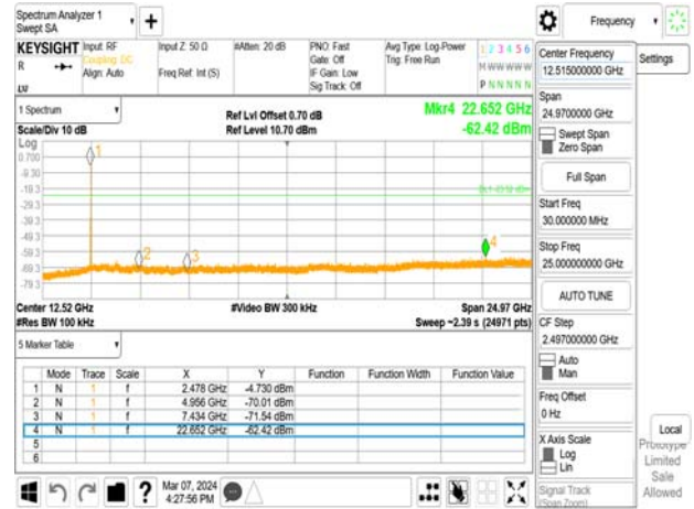
Spurious Emission_BLE 2M_HighCH38-2478MHz
