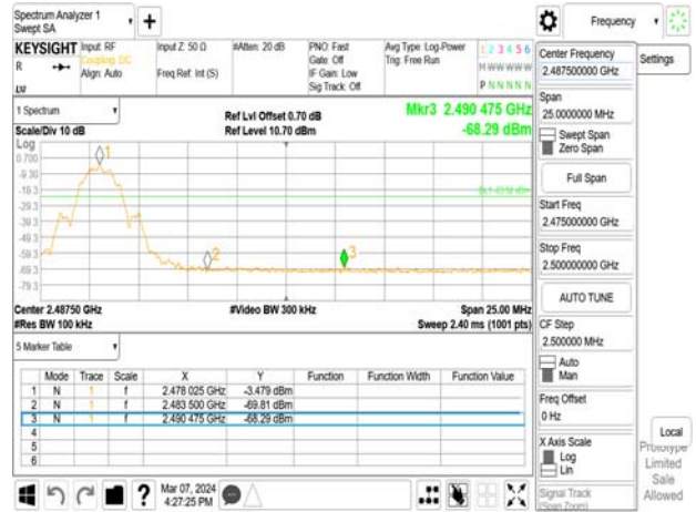
Spurious Emission_BLE 1M_LowCH00-2402MHz
