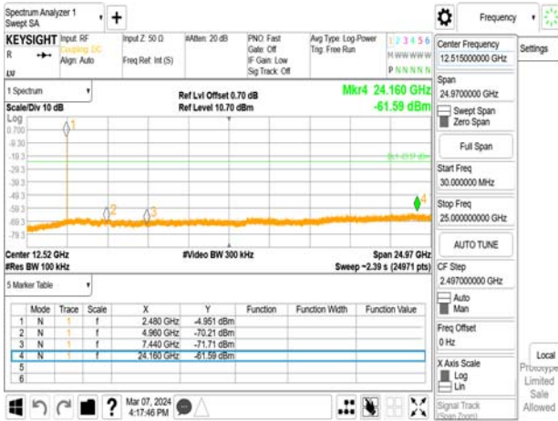
Spurious Emission_BLE 2M_LowCH01-2404MHz
