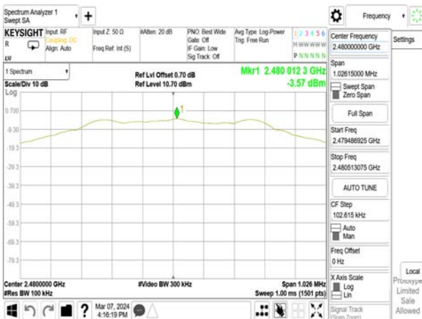
Reference Level_BLE 1M_HighCH39-2480MHz
