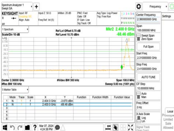
Band Edge_BLE 2M_LowCH01-2404MHz
