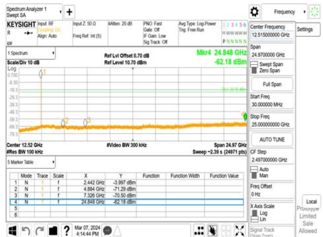
Spurious Emission_BLE 1M_MidCH20-2442MHz
