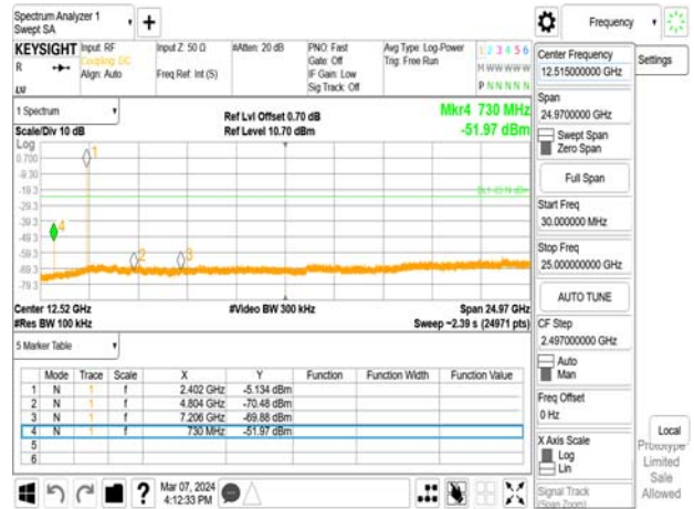
Spurious Emission_BLE 1M_MidCH20-2442MHz
