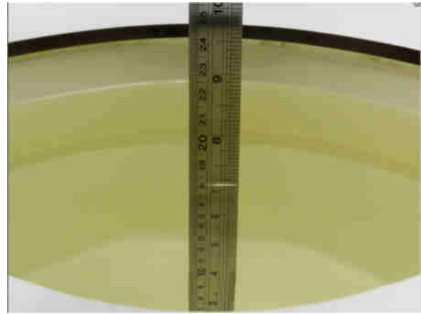
Fig 11.2 Photo of Liquid Height for Body SAR
