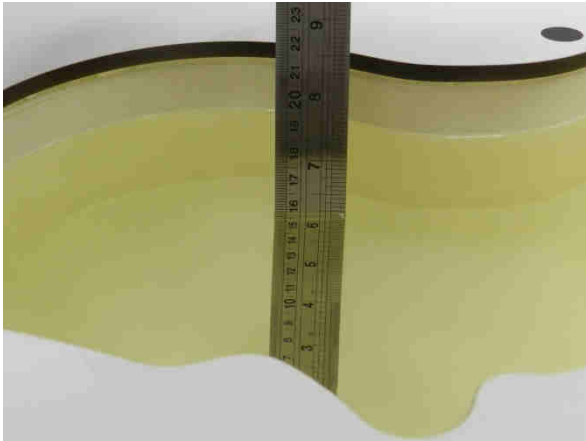
Fig 11.1 Photo of Liquid Height for Head SAR
