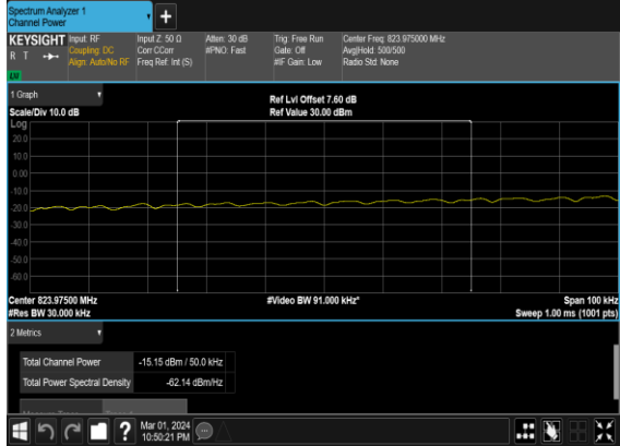
N5(5M)_DFT-s- OFDM_BPSK_Edge_1RB_Left_Low_CH CHP PASS
