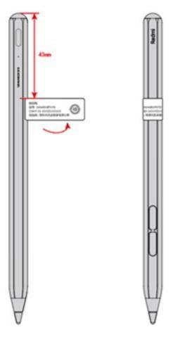
Pen body tags, labels, 43 mm from the top from a laser carving plane edge about 1 mm to the right start, not place them on the edge, counterclockwise around on pens, as shown above
