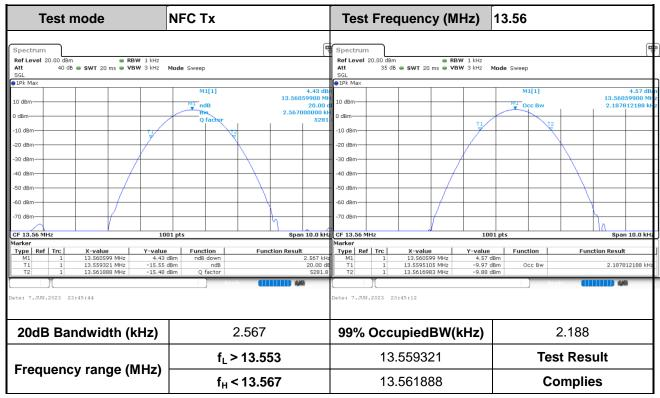
**Remark:** Because the measured signal is CW adjusting the RBW per C63.10 would not be practical since measured bandwidth will always follow the RBW and the result will be approximately twice the RBW.
