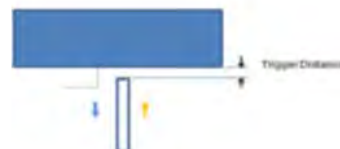
Picture : Proximity Sensor Triggering Distances Assessment(Top/Bottom Edge)
