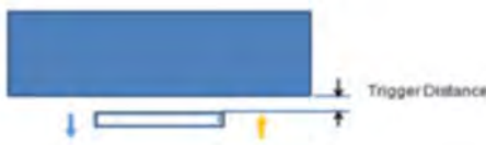
Picture : Proximity Sensor Triggering Distances Assessment(Back/Front Side)
