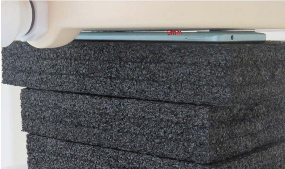
Picture 11: Back Side, the distance from handset to the bottom of the Phantom is 0mm
