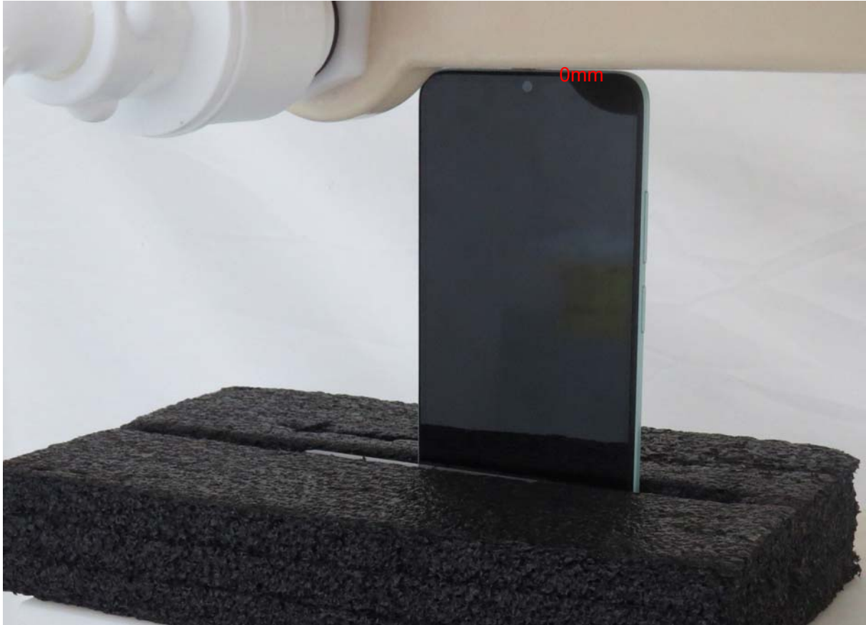
Picture 15: Top Edge, the distance from handset to the bottom of the Phantom is 0mm
