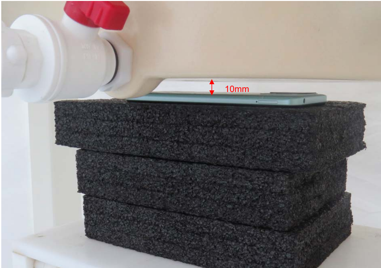
Picture 5: Back Side, the distance from handset to the bottom of the Phantom is 10mm
