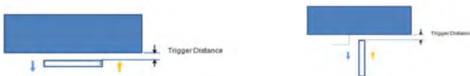
Picture : Proximity Sensor Triggering Distances Assessment(Back/Front Side) Picture : Proximity Sensor Triggering Distances Assessment(Top/Bottom Edge)
