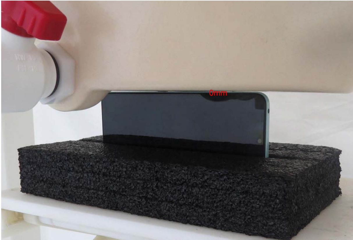
Picture 13: Left Edge, the distance from handset to the bottom of the Phantom is 0mm
