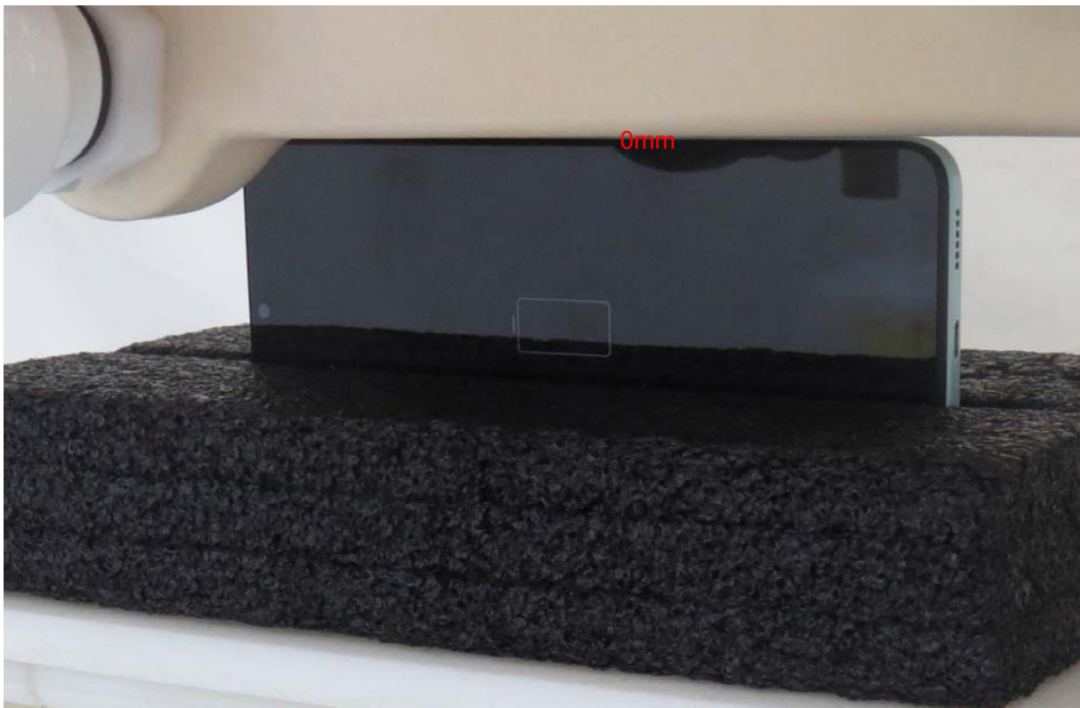
Picture 14: Right Edge, the distance from handset to the bottom of the Phantom is 0mm
