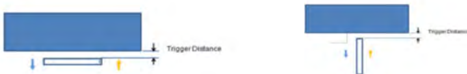
Picture : Proximity Sensor Triggering Distances Assessment(Back/Front Side) Picture : Proximity Sensor Triggering Distances Assessment(Top/Bottom Edge)
