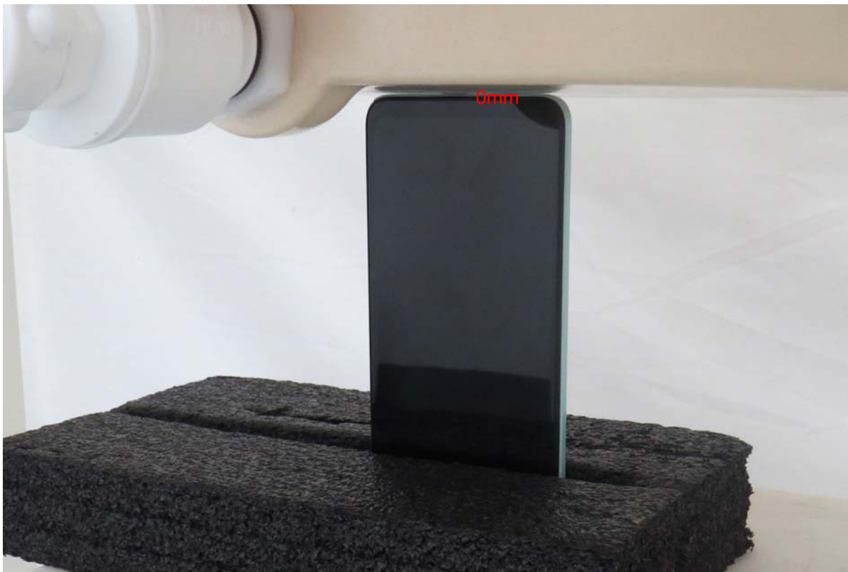
Picture 16: Bottom Edge, the distance from handset to the bottom of the Phantom is 0mm
