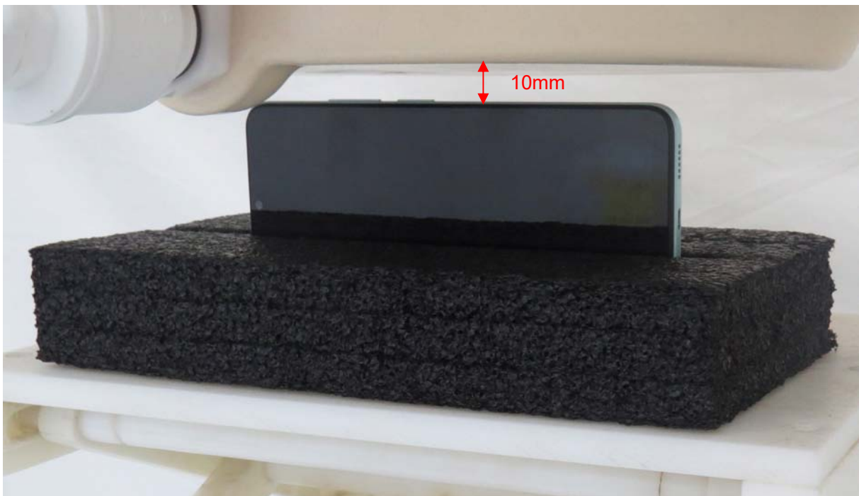
Picture 8: Right Edge, the distance from handset to the bottom of the Phantom is 10mm
