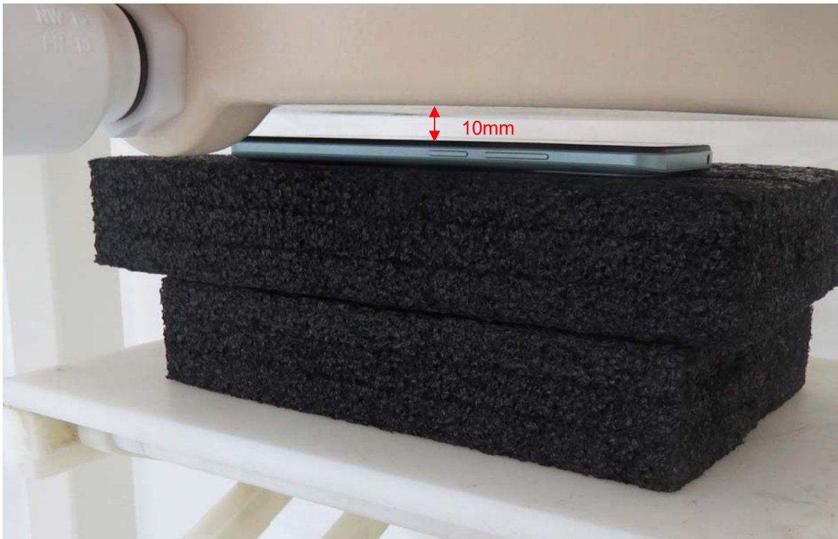
Picture 6: Front Side, the distance from handset to the bottom of the Phantom is 10mm
