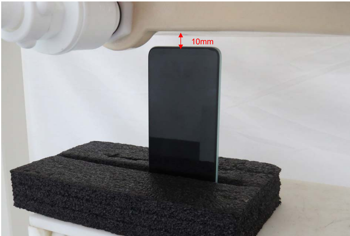
Picture 10: Bottom Edge, the distance from handset to the bottom of the Phantom is 10mm
