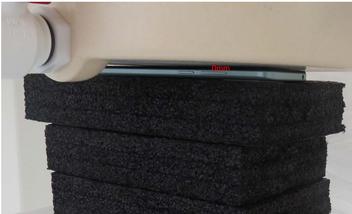
Picture 12: Front Side, the distance from handset to the bottom of the Phantom is 0mm
