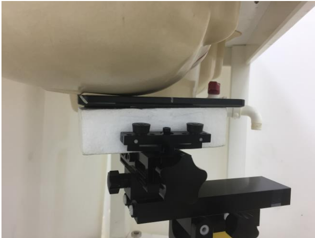
Right Cheek, Test Separation 0 mm
