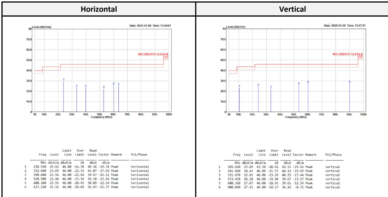
*Result = Reading + Correct Factor**Margin = Result - Limit**Correct Factor = Antenna Factor + Cable Loss - Amplifier Gain**Spurious emissions more than 20 dB below the limit were not reported*
