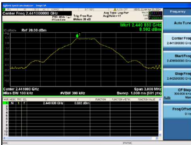
GFSK MIDDLE CHANNEL, CARRIER LEVEL
