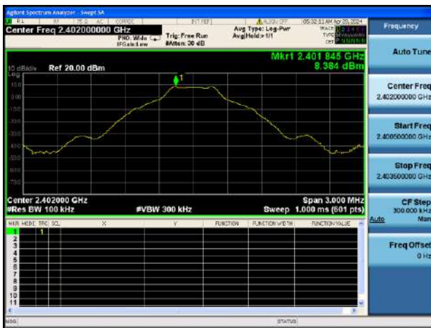
GFSK LOW CHANNEL, CARRIER LEVEL
