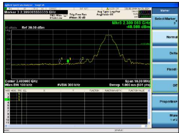
GFSK LOW CHANNEL, BAND EDGE
