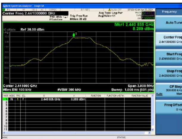
GFSK MIDDLE CHANNEL, CARRIER LEVEL
