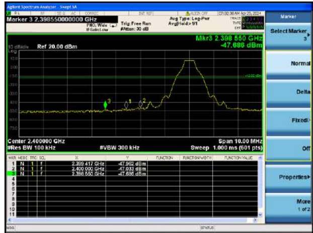
GFSK LOW CHANNEL, BAND EDGE
