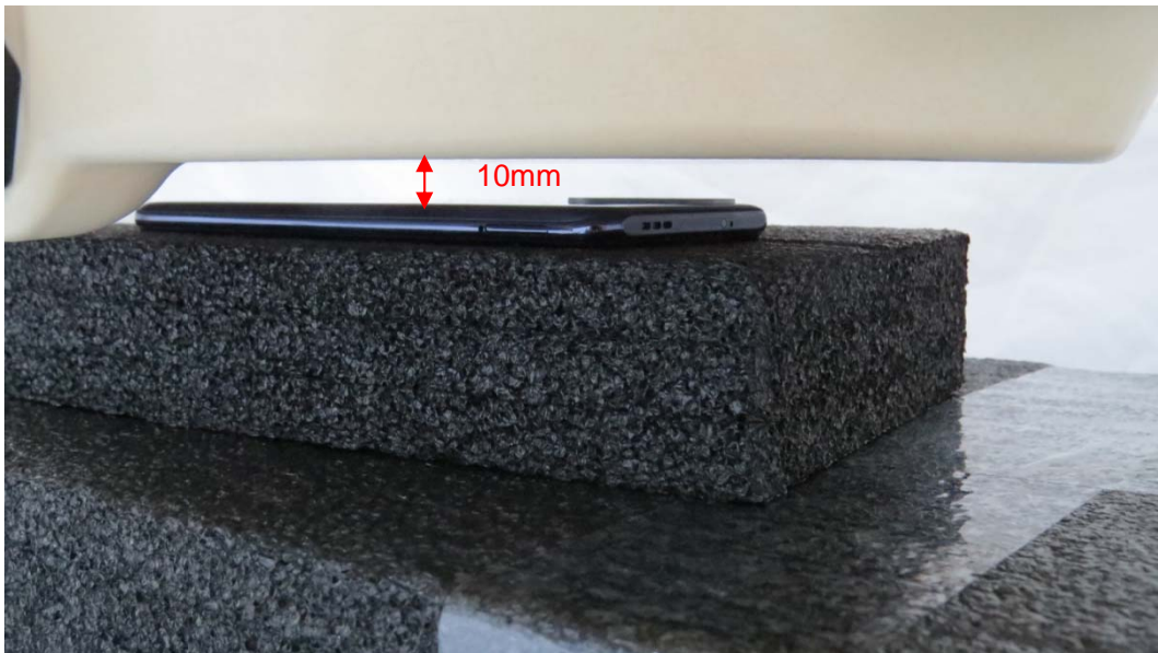
Picture 8: Back Side, the distance from handset to the bottom of the Phantom is 10mm
